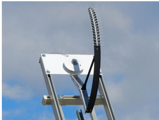
Figure 3. Diffuse POA irradiance measurement for elevation-only rotations
