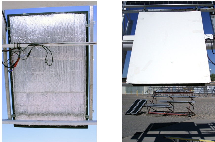
Figure 5. Module prepared for thermal test. Insulated back surface (left) and module shade (right).
