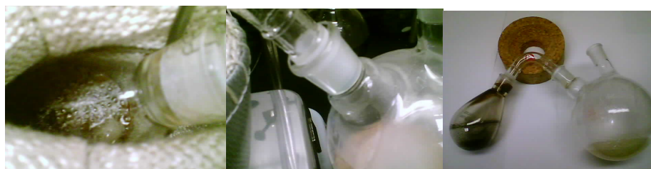
Figure 4. Reaction set up for thermolysis of pure PHB. Left panel, heating of flask containing PHB. Middle panel, top of receiving flask. Right panel, flasks after conclusion of experiment.
