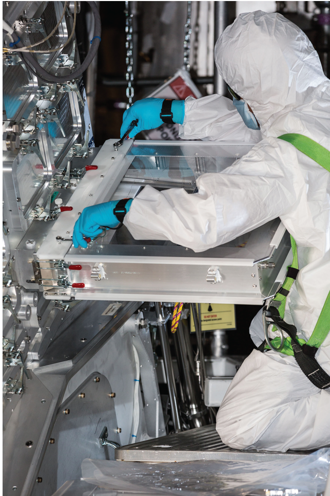
Fig. 118 Close-up view of an FOA optic exchange
