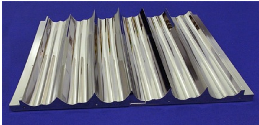
Figure 80: Aluminum sheet involutes used behind flashlamps of the large 1\omega amplifiers.
