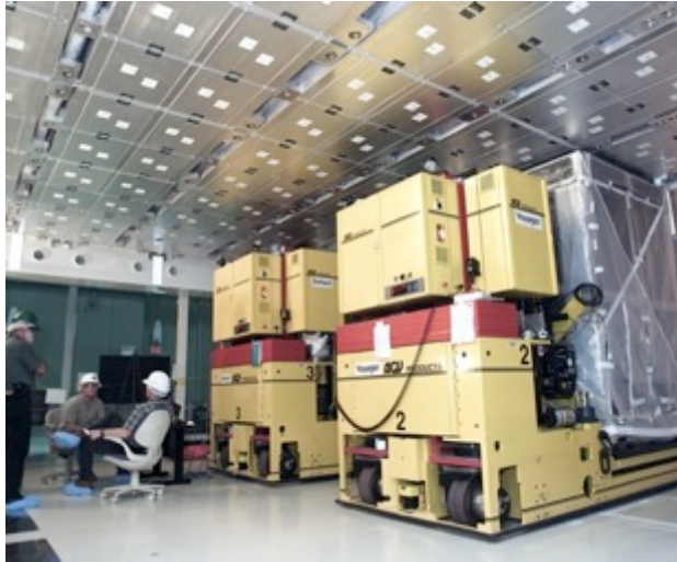
Fig. 13: Laser slab cassettes are transported into the laser bay and inserted into the beam path using special portable cleanrooms carried by autonomously guided vehicles (AGVs). 44
