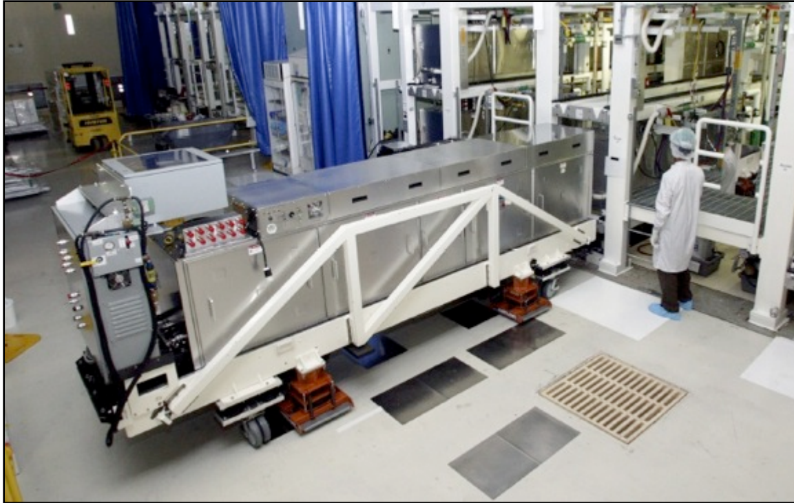
Fig. 41: A photograph of a PAM LRU being readied for installation in the region below the Transport Spatial Filters. The two sides of the PAM, seen earlier in Fig. 29, the regen and the four-pass preamplifier, are supported back-to-back to each other in the LRU.
