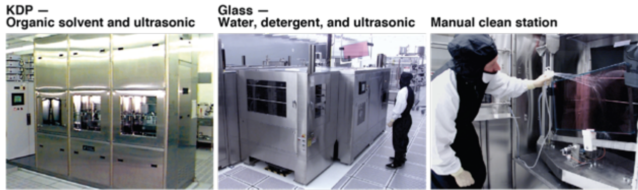
Fig. 54: OPF stations for cleaning incoming optics.
