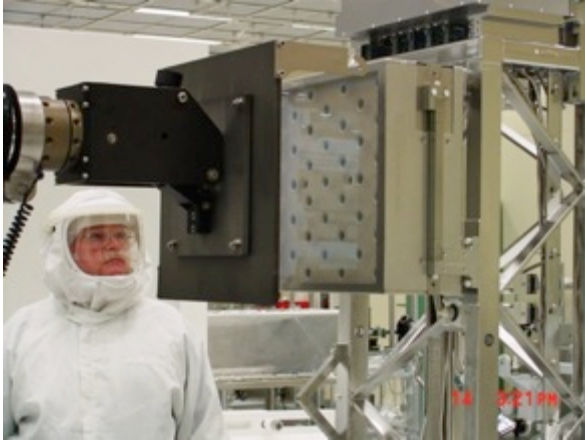
Fig. 58: An LM1 being loaded into its LRU. The deformable mirror actuators can be seen through the coated surface of the mirror that is highly reflective at 1\omega , yet transparent in the visible.
