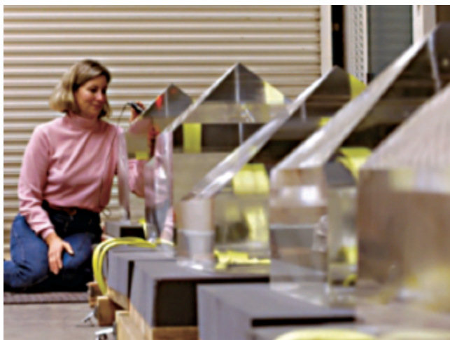
Fig. 97: Large KDP crystals awaiting further cutting and finishing for use as polarization rotators or frequency doublers in NIF. As production began, Ruth Hawley was the group leader for KDP Rapid Growth/Pilot Production.
