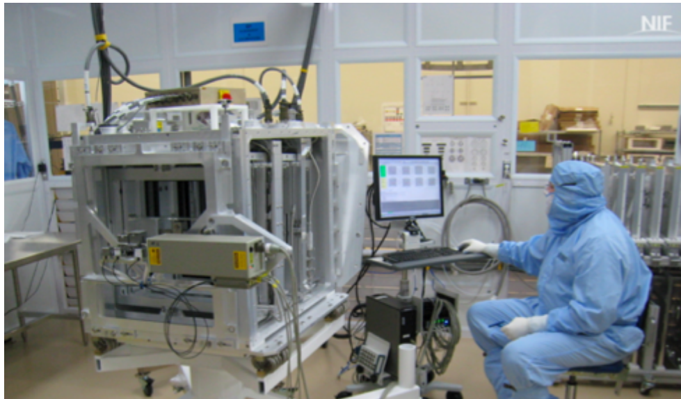
Fig. 88: Assembly of production FOA integrated optics modules in a temporary factory set up at LLNL.
