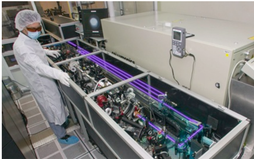
Fig. 100: The SNL \sim 500 ps laser developed for off-line conditioning of tripler crystal optics for NIF, with its developer, John Honig.
