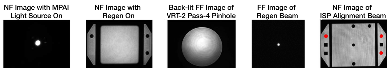
Fig. 130: Near- and far-field ISP images used for centering and pointing of the 1 Hz regen beam and for co-alignment of the ISP cw alignment beam with the pulsed regen beam (Ref. 185).
