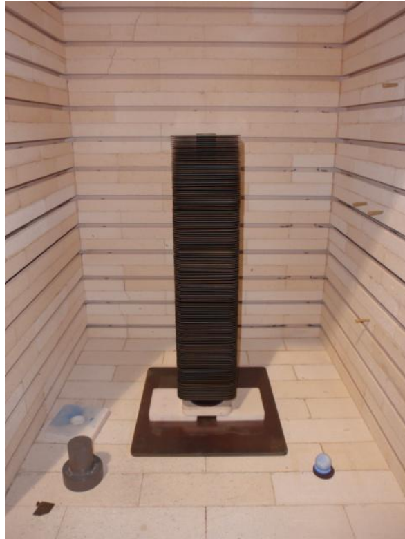
Figure 2.2.11 – One of the first 1-TPD modules made entirely from Advanced Architecture wafers in the assembly furnace.
