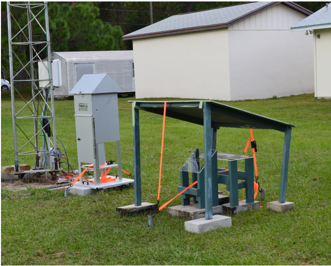
Fig. 2. Set-up used for collection of samples in this experiment. On the left is the TSP filter sampler, and on the right is the deposition coupon deployment structure.
