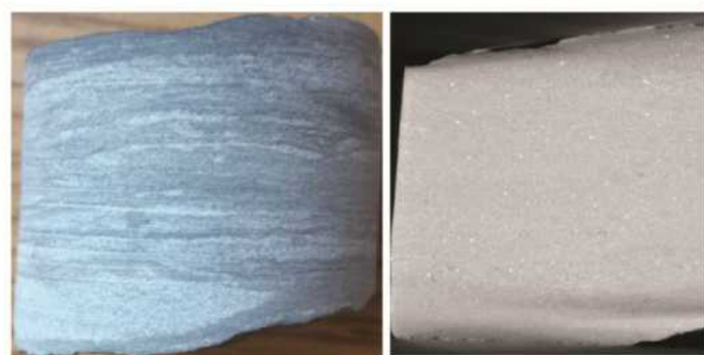
Figure 13. Above. A one-inch diameter core sample (left) and cross sectional micro-CT image (right).
