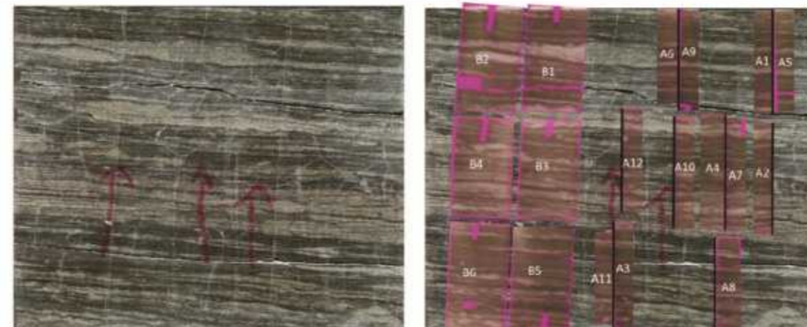
Figure 5. Left. Left scan is of front face of slice 2. Right scan is the same and includes location of thin section cut from slice 1 compared to slice 2. Thin section A1-A12 were cut perpendicular to slice 1 and 2. The position of these perpendicularly cut thin sections are represented with a scan of the right or left side of the thin section according to the side of the thin section that was originally closer to slice 2. This side is marked with a black line. Thin sections B1-B6 were cut parallel to slice 2.
