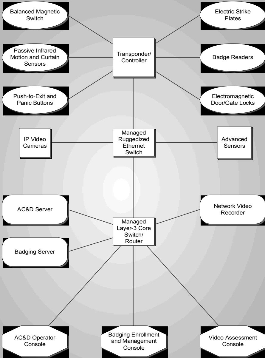
Physical protection system (PPS) hardware and networks can be abstracted at layers.
