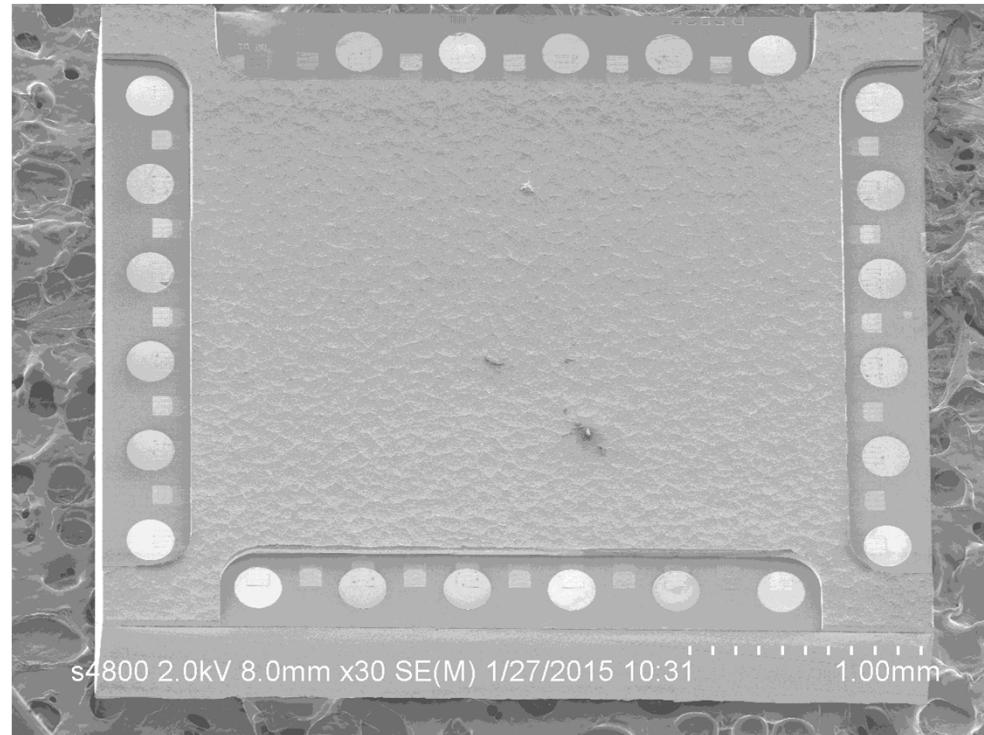
The dies are then singulated using a low water flow dicing saw.
