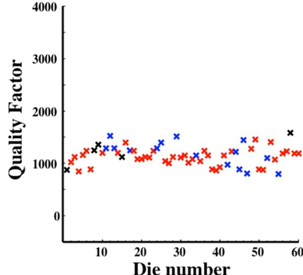
22 MHz resonator – the low frequency makes this device very sensitive to package pressure. Of 60 die, 6 were non-functional, 4 had spurs on resonance, 17 had high Q's indicating vacuum, and 33 were low vacuum or atm.
