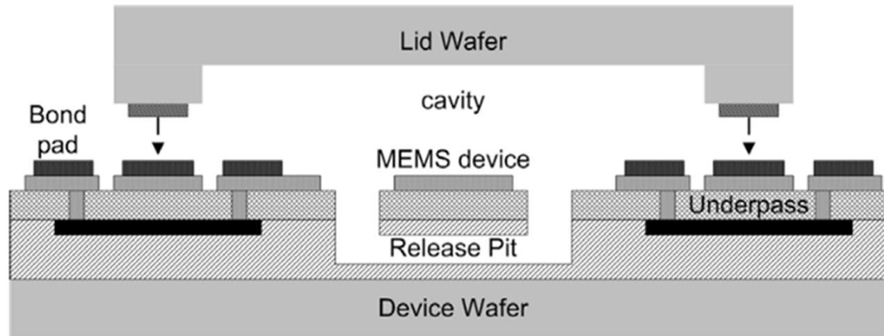
Fabrication sequence is, then, make a die and lid wafer in a CMOS factory, move to a  $\mu$ fab for post processing. This includes Au/NiV metal deposition and patterning, wafer level  $\text{XeF}_2$  release, wafer bonding under vacuum, plasma back etch of the lid, auto-probing and RTA frequency trimming, and balling.
