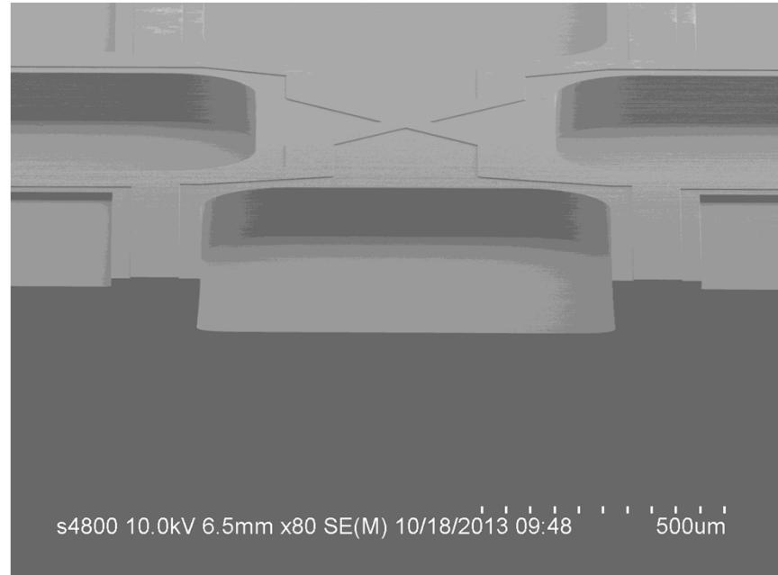
Lid wafer is made using 3 different silicon etches, thermal oxidation, and a-Si uniform deposition.
