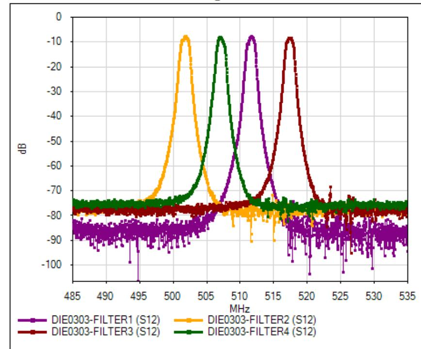
Although other types exist, the Lamb wave acoustic resonator is interesting because the thickness is thin film ( $\sim 750$  nm) yet can accommodate different frequency devices all set by the lithography. Frequency range can be low (few 10's of MHz) or high ( $> 3$  GHz).
