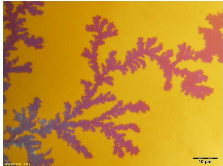
Bonding induced recrystallization of PECVD a-Si. Although the Au was restricted to the bonding seal ring, the aSi was coated over the full lid wafer.
