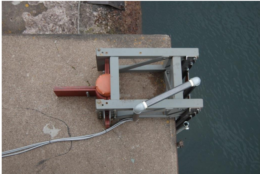
Figure 5.3(b) Top view of the bollard (orange), bollard collar (darker orange), deck and vertical frames (gray) shown supporting the ice force measuring plate. The vertical and horizontal piping encases the data cabling which can be seen on the deck leading from the IFMS to the data logger.
