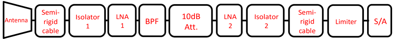
Figure 7. Block diagram of the wideband autocorrelation radiometer.
