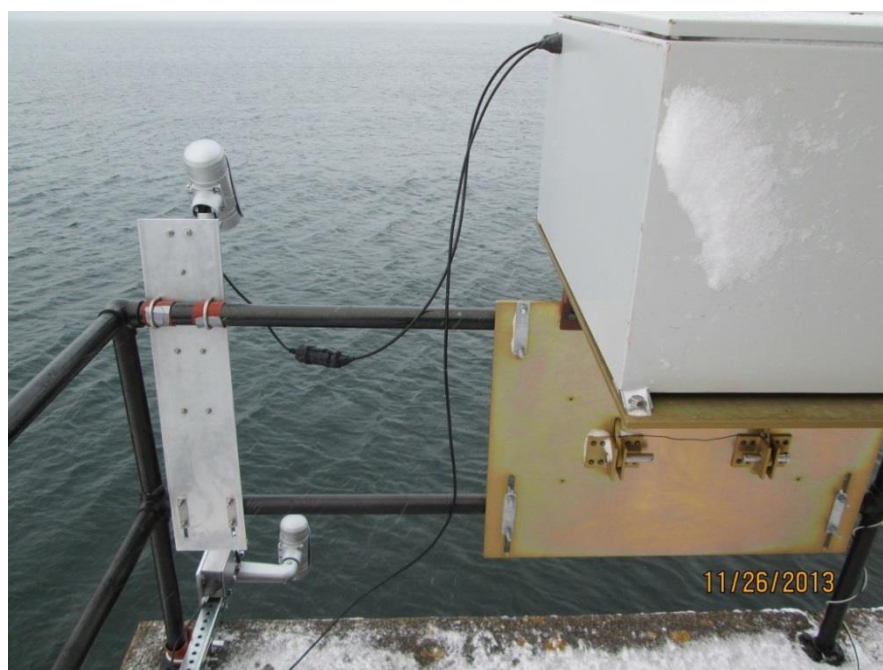
Figure 7.3. Photo showing left stereo camera (upper left) and IFMS camera (lower left).
