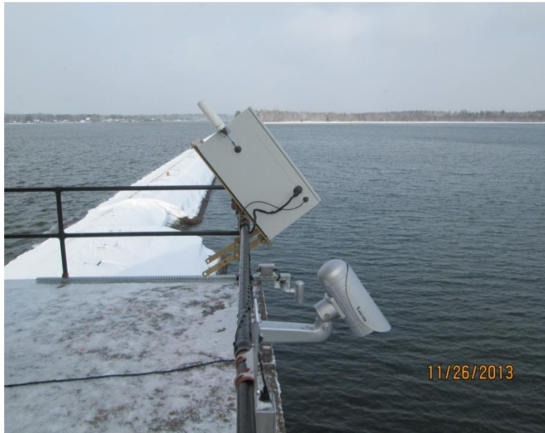
Figure 6.1 (a) WiBAR as it is pointed to ‘view’ the water surface (b) WiBAR antenna opening, protected by water-proof radome (c) WiBAR with one of the Scene Capture System cameras in the foreground.
