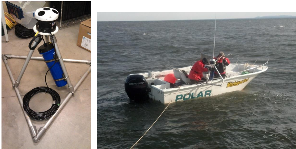
Figure 8.1. (a) AWAC in custom tripod stand (b) MTU GLRC team deploying the AWAC to the east of the experimental site.
