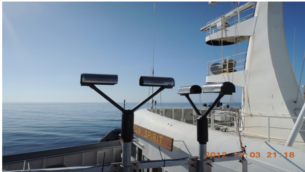
Figure 1. The two Parsivel disdrometers on the Horizon Spirit set perpendicular to each other to mitigate the impact of wind direction on the measurements of rainfall and raindrop particle size distribution.
