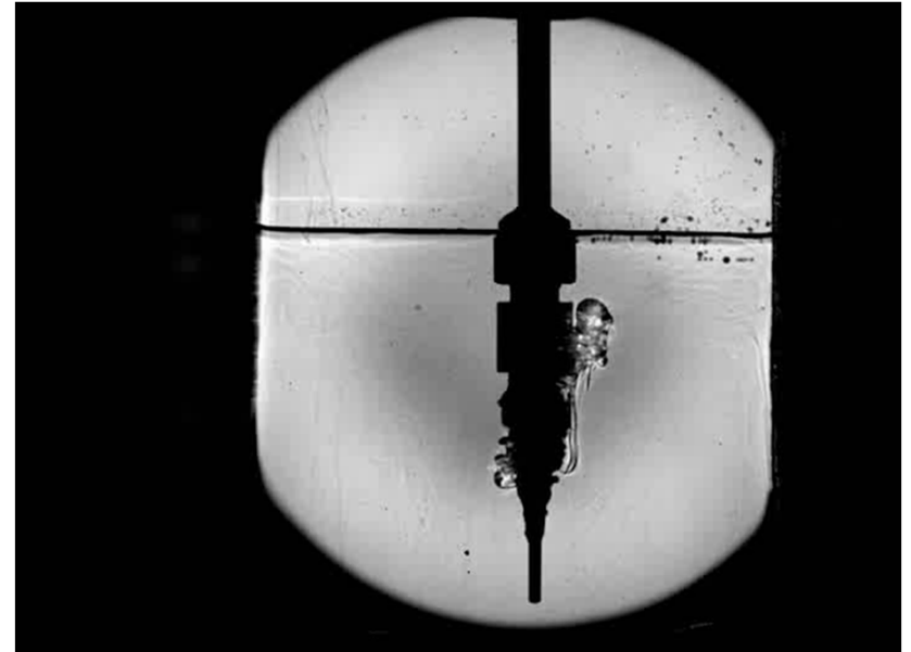
Nozzle near air-brine interface
