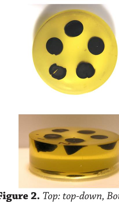
Figure 2. Top: top-down, Bottom: side view of cross-sectioned o-rings embedded in epoxy.
