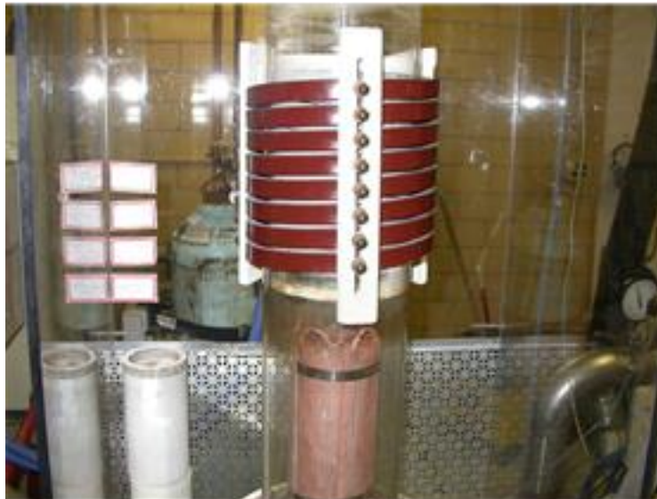
Figure 17: Induction furnace used for liquid metal extraction experiments
