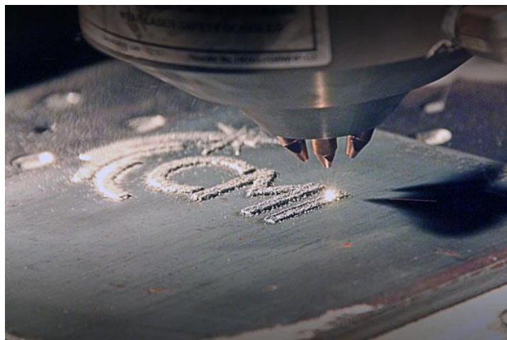
Figure 28: The Ames Laboratory/CMI LENS MR-7 3D additive manufacturing system to streamline the process of bulk combinatorial materials research, producing a large variety of alloys in a short amount of time
