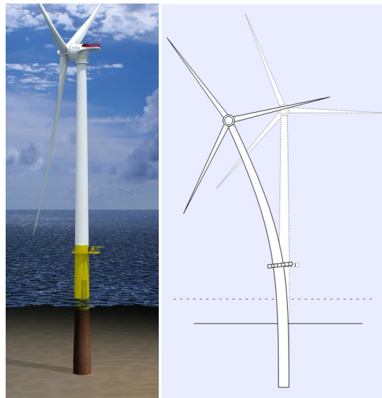
Figure 2 – GE Haliade150-6MW on a Monopile and 1 st bending Side-to-Side mode in a Monopile fixed-bottom substructure (Mark L. Brodersen, 2014)
