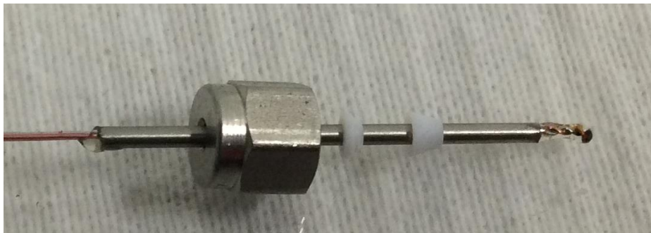
Figure 3-17: Thermocouple with tubing, epoxy, and ferrules
