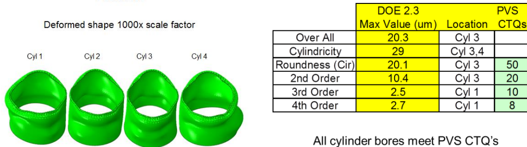
Figure 89 - Bore distortion analysis.
