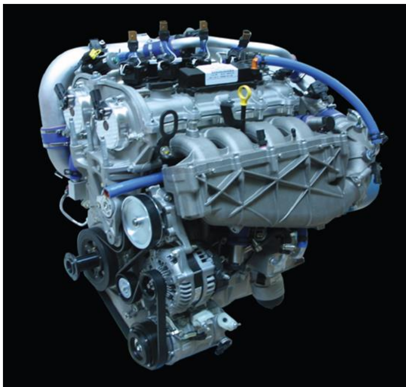
Figure 7 - 2.3L GTDI DOE engine.
