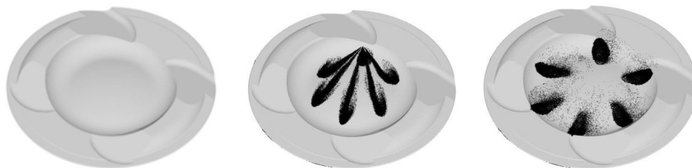
Figure 19 - Piston top showing fuel spray jets at 35^\circ bTDC (middle) and 30^\circ bTDC (right).
