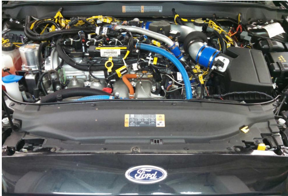
Figure 212 - 2.3L engine with measurement instrumentation installed in a Fusion vehicle.
