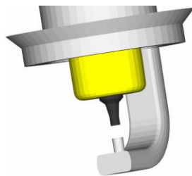
Figure 117 - Spark plug firing end detail.
