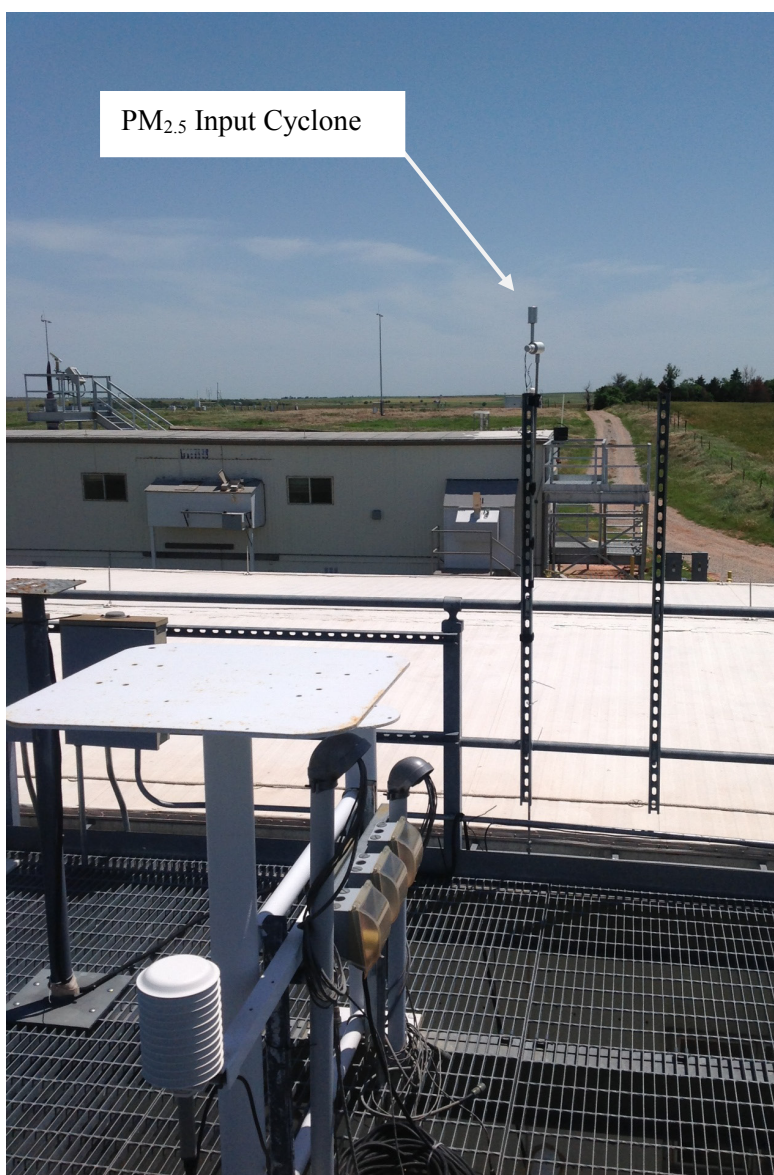
Figure 2. Inlet tubing for carbon sampling at the SGP site. The PM 2.5 input cyclone is installed at the top end of the tubing.
