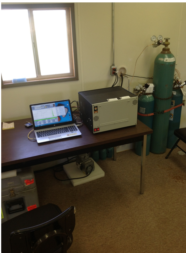
Figure 1. Operational computer for the carbon sampling system at the Southern Great Plains site.
