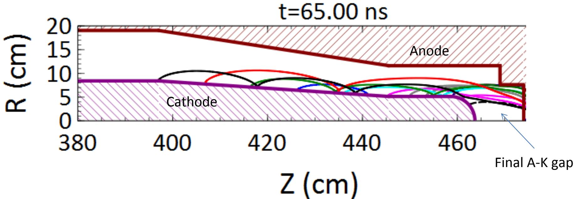
LSP simulations indicate that the emittance decreases as the electrons are accelerated across the final A-K gap
