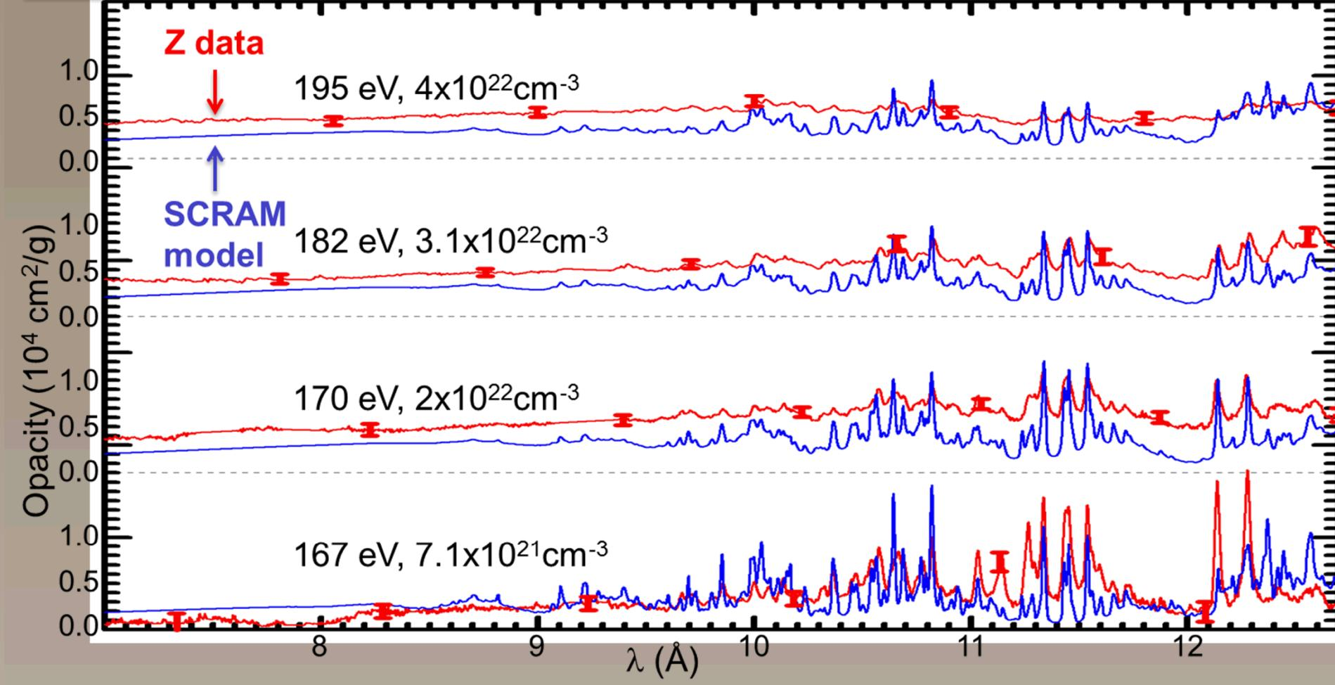
At high temperature, density, calculations are generally lower than the data
