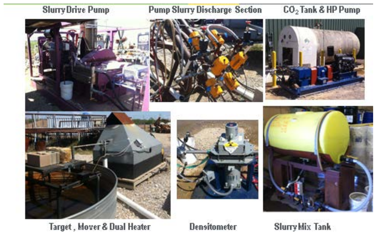
Figure 28. Clockwise-Freemyer slurry drive water pump, HPSP#4 control valves, AirGas CO 2 Tank, Bear CO 2 pump, dual NorthStar heaters, ThermoFisher densitometer, polymer mixing tank
