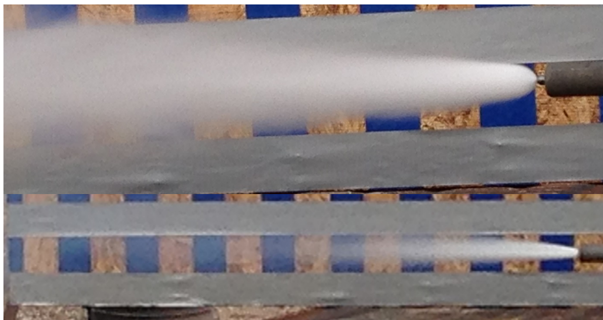
Figure 24. Spray Pattern Testing March 2013 - 2" patterns behind spray. Top-Good Wide Cut. Bottom, Test 248b-Poor Narrow Cut.
