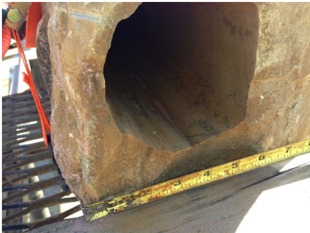
Figure 64. Exit wound due to flow choking
