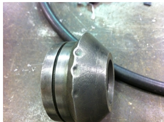
Figure 37. HPSP1 Valve Damage due to Cavitation.
