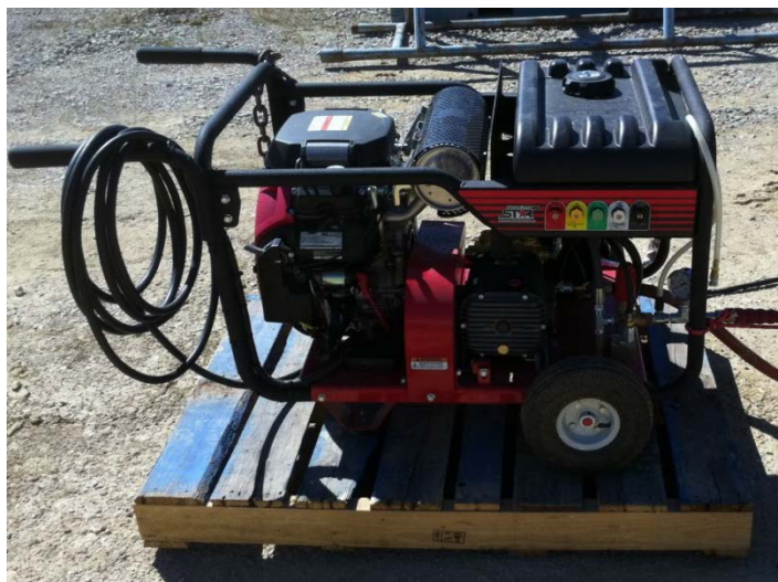
Figure 27. Small 5gpm and 5000psi 25hp water jet sprayer used for some steam tests.
