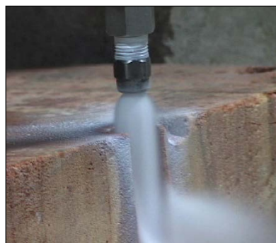
Figure 4. Drilling sandstone using 5,000 psi FLASH ASJ™ at MS&T (24)
