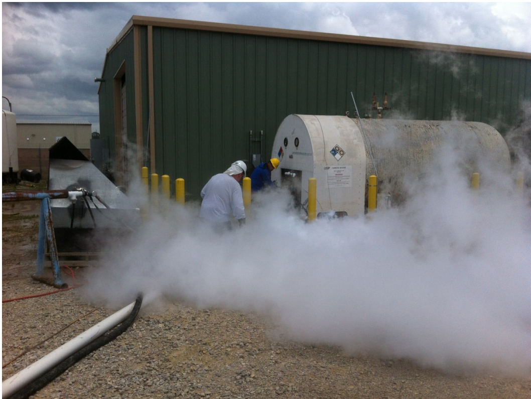
Figure 23. Bear CO 2 pump and lines cool-down procedure before testing in June 2012
