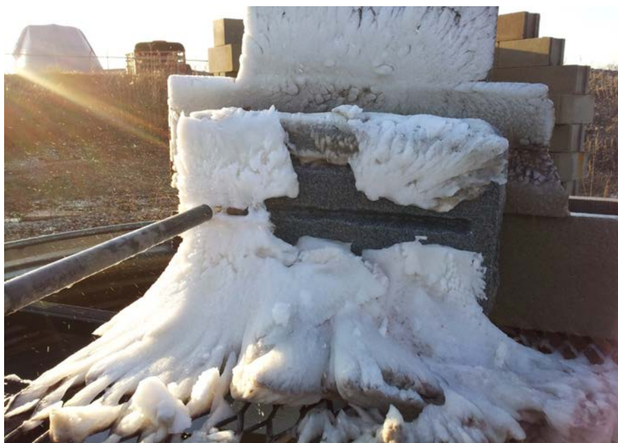
Figure 38. Icing at High Gas: Slurry Ratio Tests, if not heated-May2013 tests
