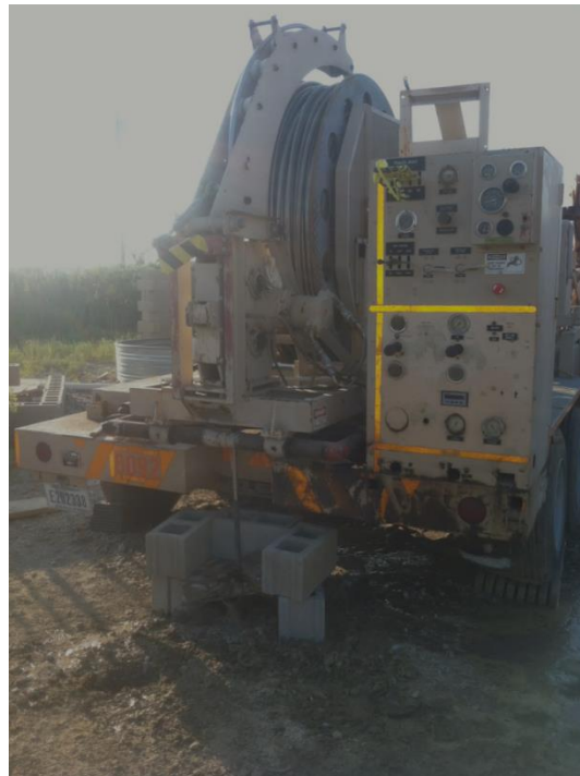
Figure 33. LANL Coiled Tubing Rig with new 1.0" high alloy steel CT
