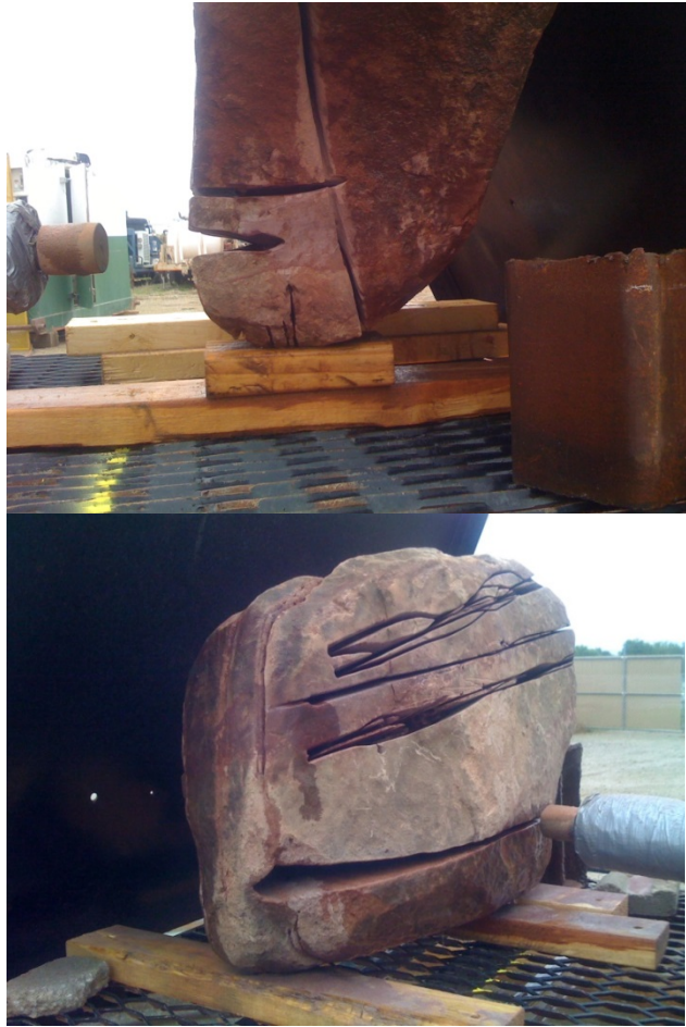
Figures 42, 43 and 44, clockwise. Steam FLASH ASJ cutting on sandstone May 2010. Showing deep tapered cuts with standard nozzles; variable stray cuts due to partial nozzle plugging; standoff effect with higher standoff (distance from nozzle to target in a gas) showing a wider cut.
