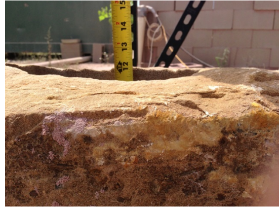
Figure 32. Use of a 3 Nozzle Bit with CO 2 FLASH. Measuring cut depth.
