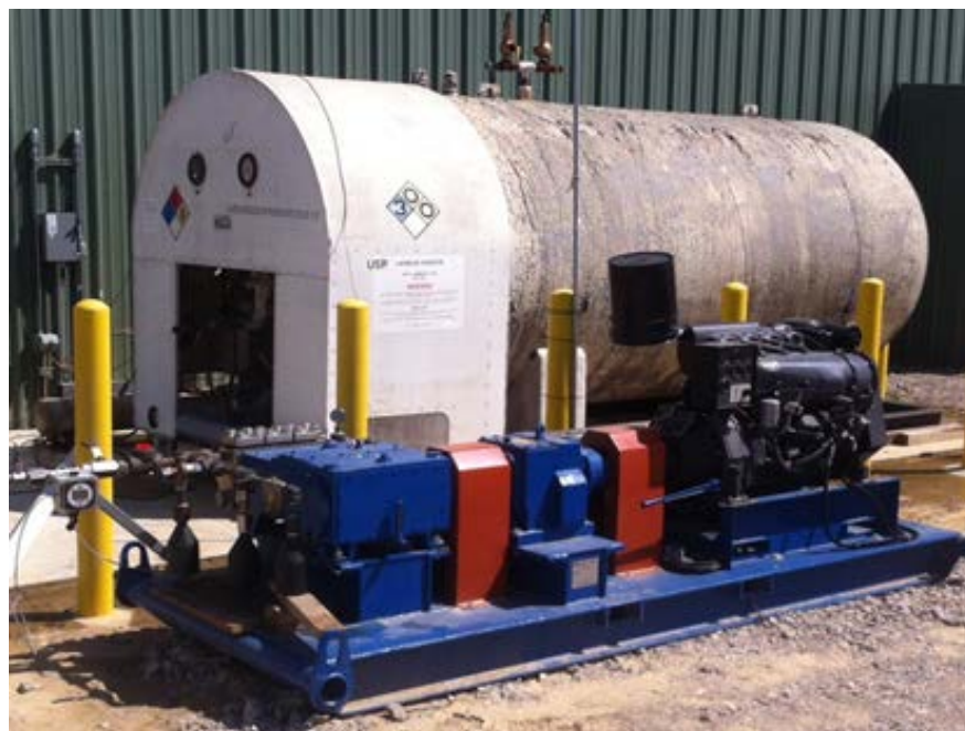
Figure 25. AirGas CO 2 storage tank, Bear triplex pump skid, charge pump and header
