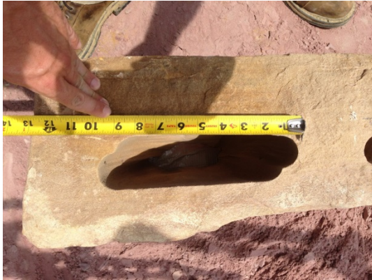
Figure 31. Three Nozzle CO 2 Bit FLASH Cut through Rock. Measuring back side hole.
