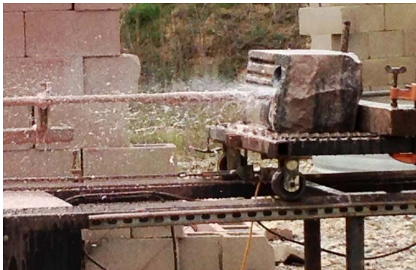
Figure 30. FLASH ASJ Drilling Hole in Granite Block on bench target mover - Spring 2013
