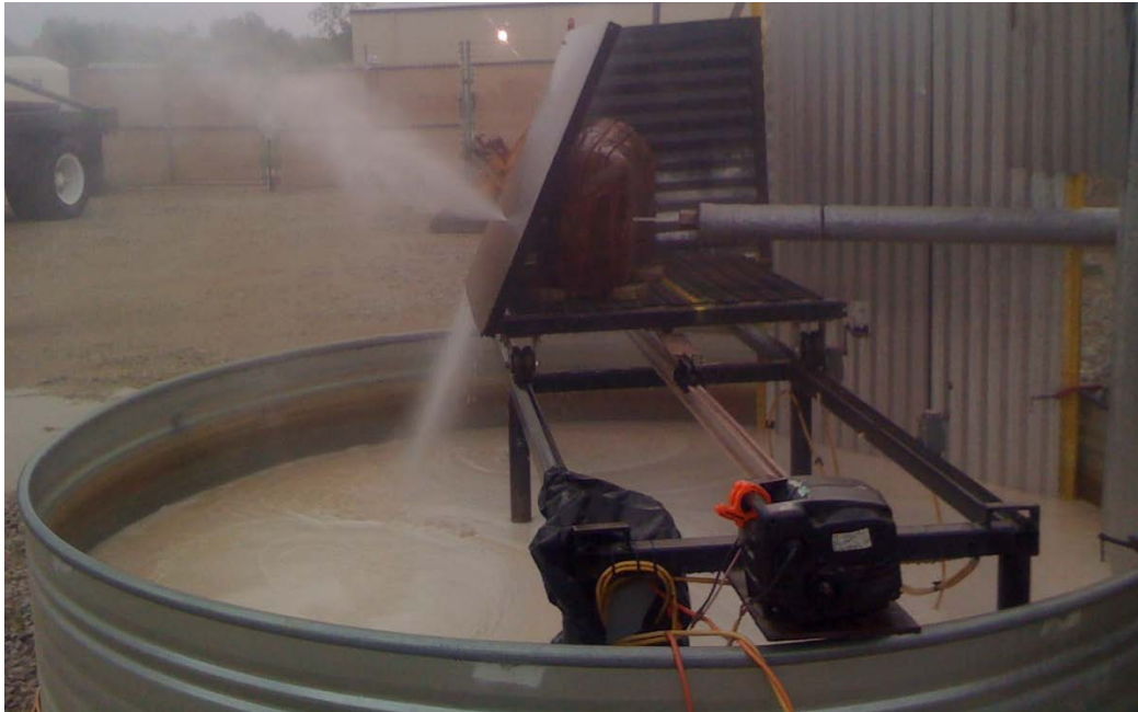
Figure 40. Steam FLASH ASJ Cutting and Boring, May 2010. Cutting through the back steel.
