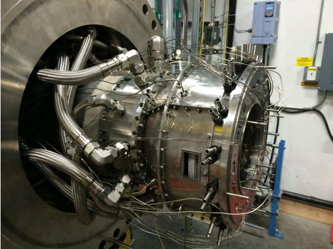
Figure 11.9: Combustor Assembly prior to hookup of fuel, air, water, and instrumentation in Redmond Lab.
