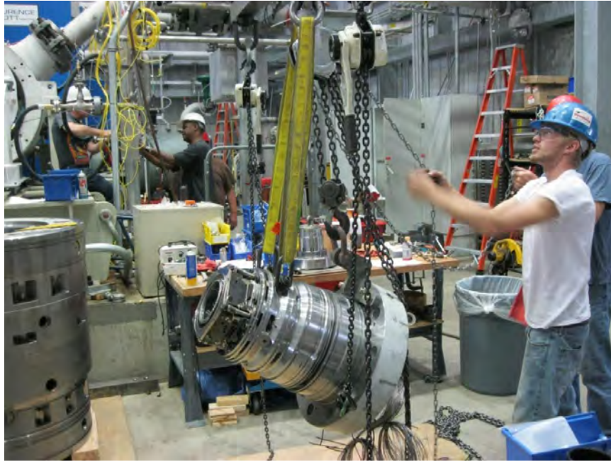
Figure 6.3: Ramgen personnel assembling the bundle.
