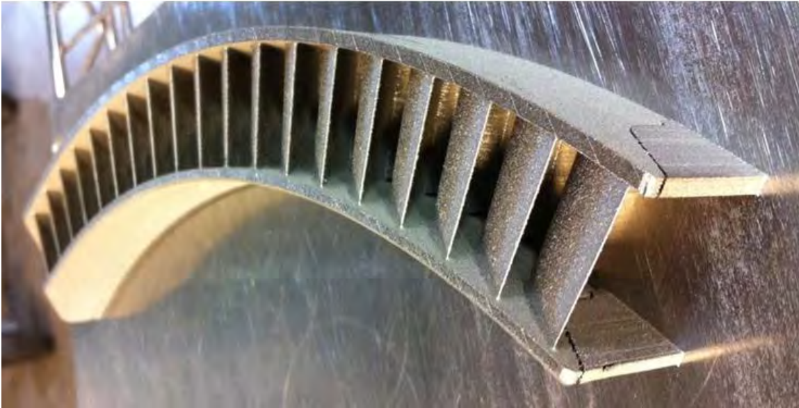
Figure 11.27 - View of the as-printed trailing edges on the cobalt chrome replacement part.
