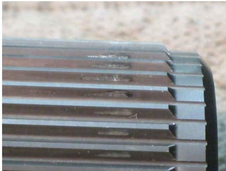
Figure 7.18: HS coupling spline wear marks
