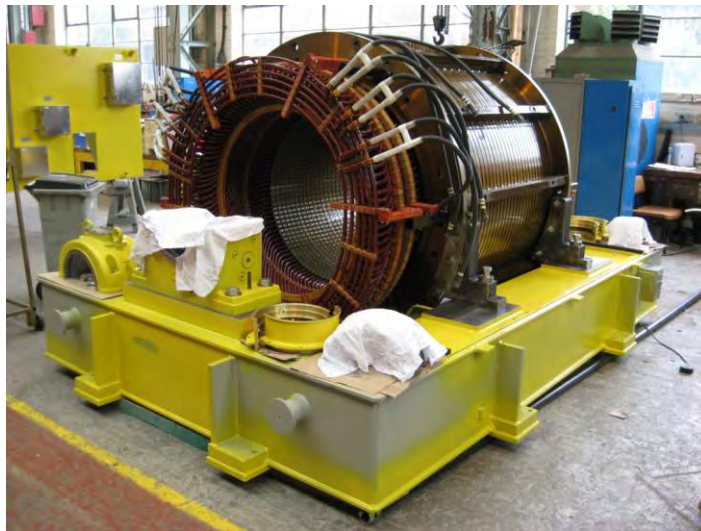
Figure 7.1: Partially Assembled Typical 10 MW Motor Showing Base Frame and Stator
