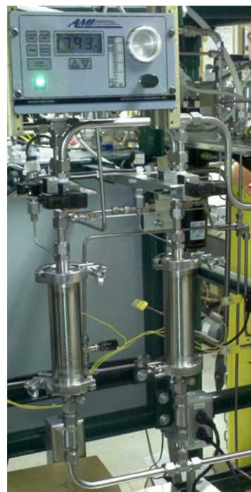
Figure 27. Picture of TDA's two bed VSA cycle test system.
