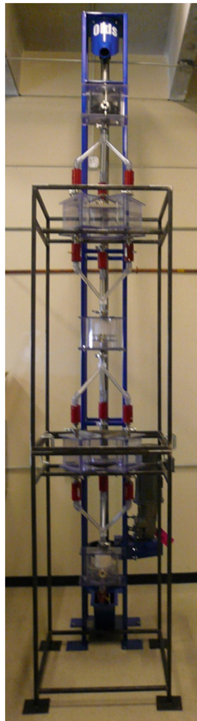
Figure 56. Picture of cold flow visualization moving bed system fabricated by TDA.
