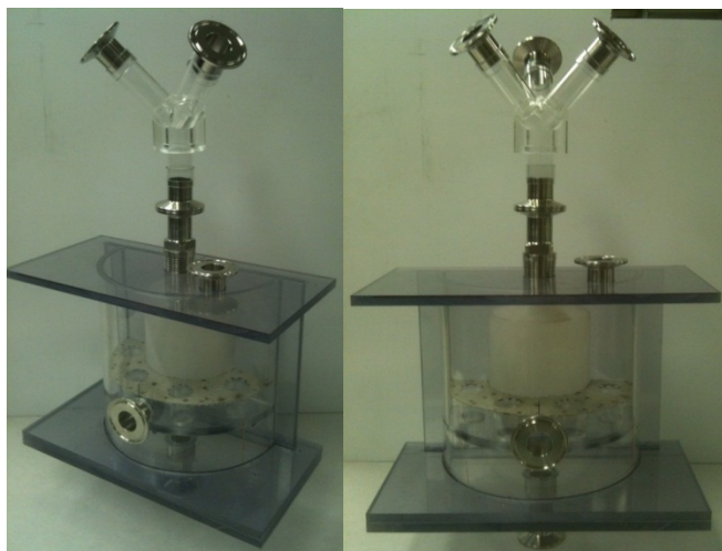
Figure 49. Clear adsorption reactors with lock hopper inlets
