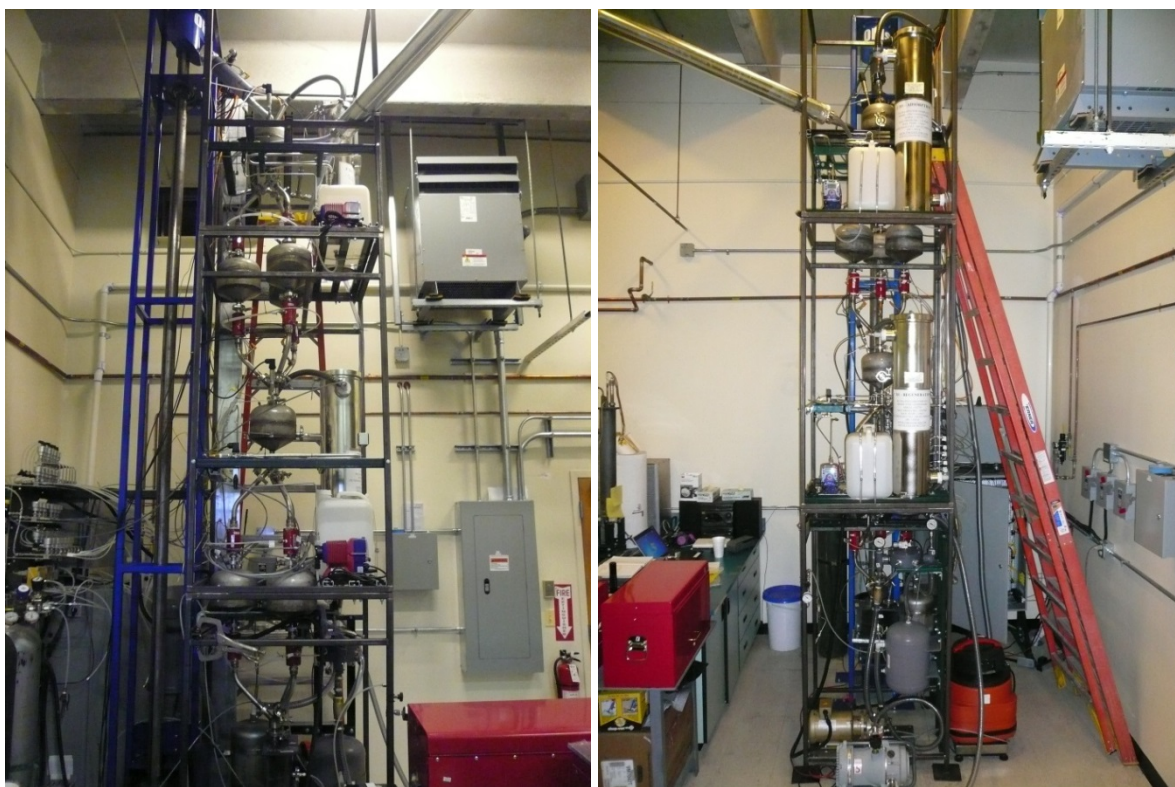
Figure 58. Picture of prototype moving bed system fabricated by TDA.
