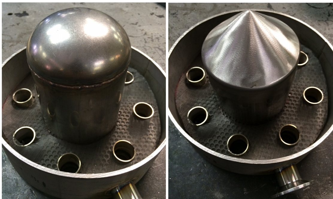
Figure 61. Reactor internals rounded top – old (left) and conical top – new (right).
