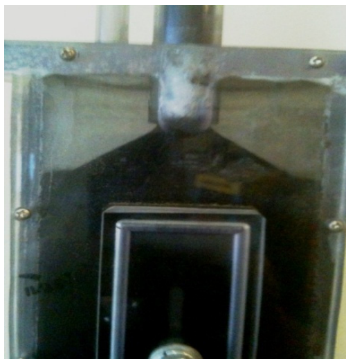
Figure 51. CO 2 sorbent flowing through clear mini reactor
