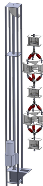
Figure 53. Solid Works rendering of the Adsorption, regeneration, and the purge reactors along with the lock hoppers.
