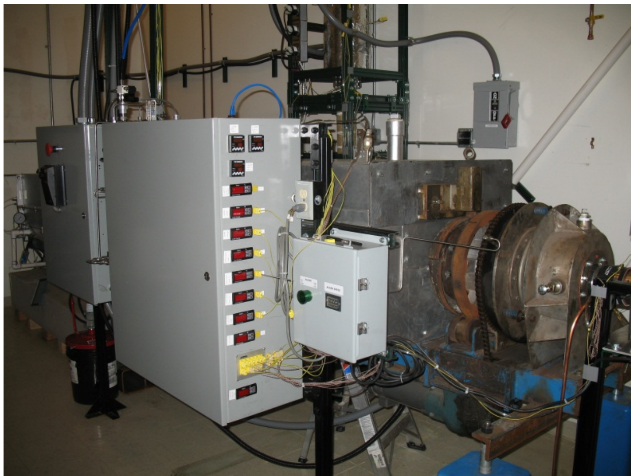
Figure 57. TDA's 7" rotary kiln used to produce the sorbent used in the prototype unit field tests.
