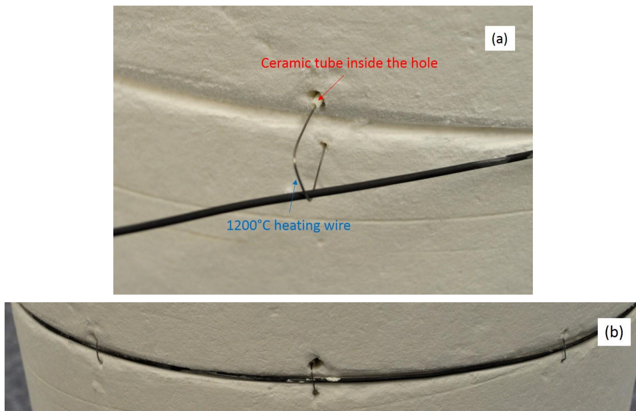
Figure 11-20. Inconel tube mounting on the thermal insulation layer.
