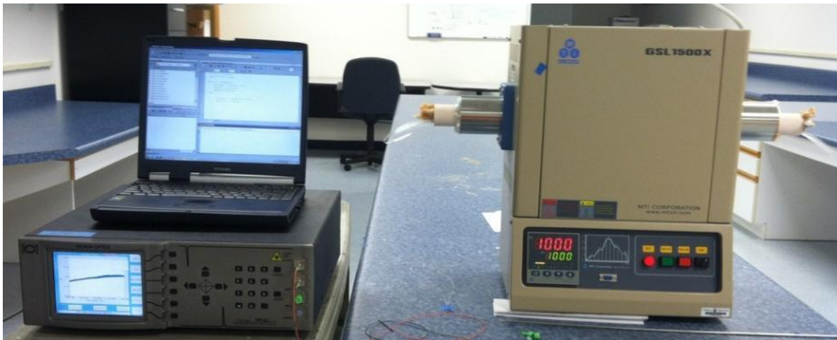
Figure 9-9. Experiment setup to measure the transmission degradation of SMF28 at 1000 °C.
