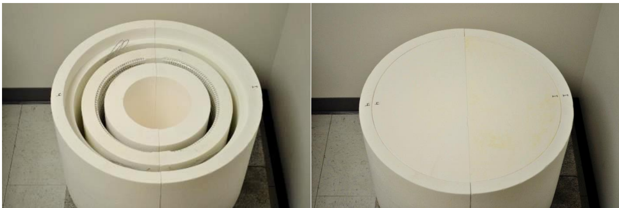
Figure 11-16. Assembled double-layer furnace.
