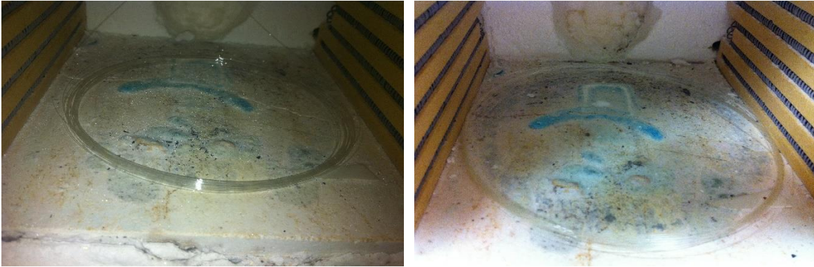
Figure 9-14. Photos of 10 cm diameter coil of 10 m long SMF28 fibers with (left) and without (right) internal twisting stress.
