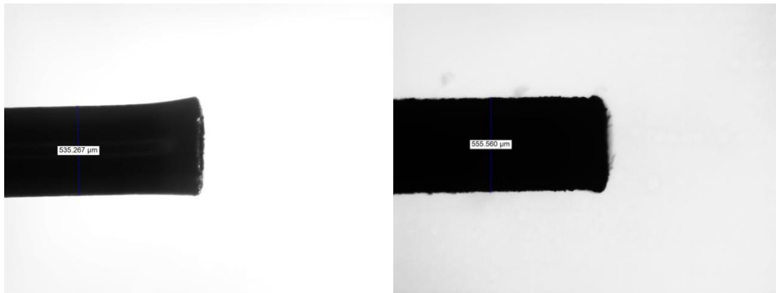
Figure 10-2. Microscope picture of stainless steel tubing before (left) and after (right) annealing.
