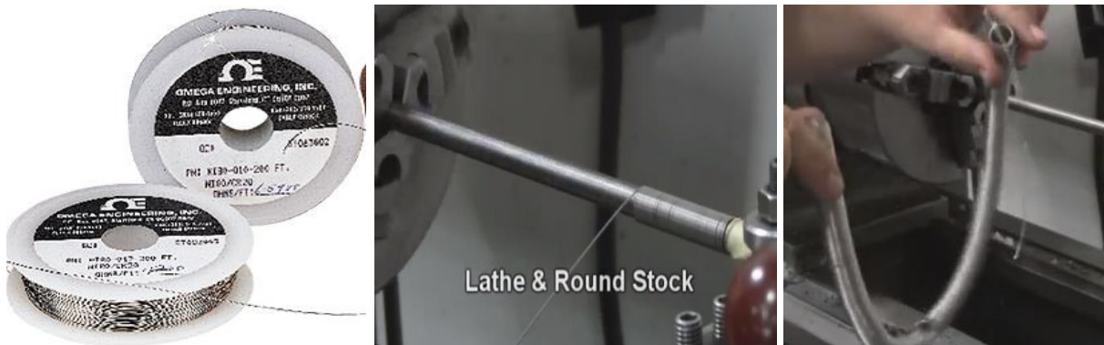
Figure 11-8. Heating wire winding. [63, 64]
