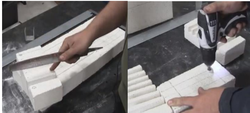
Figure 11-7. Refractory bricks milling. [63]
