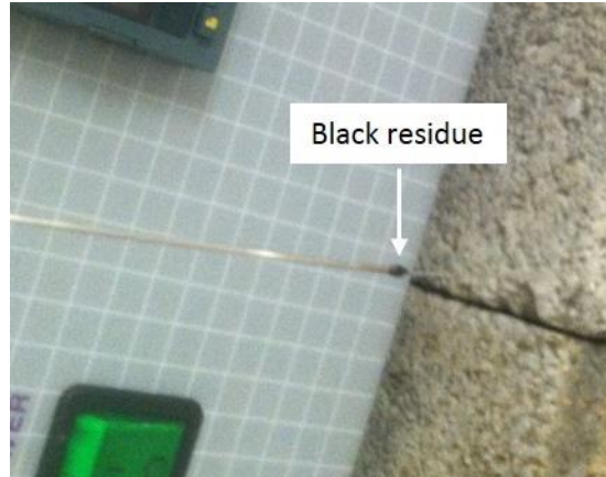
Figure 10-6. Black residue observed on the fiber near one of the tube outlets.
