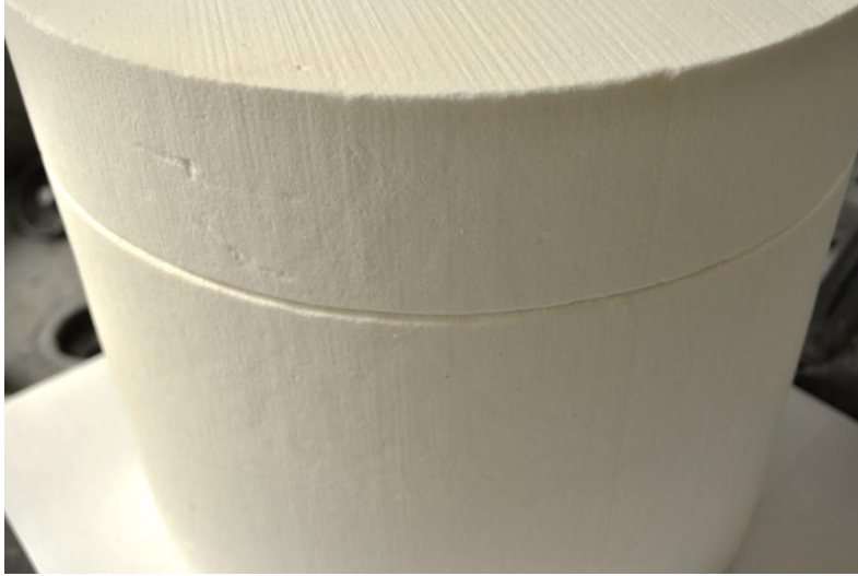
Figure 11-18. Sensor positioning groove carved on the inner insulation layer.
