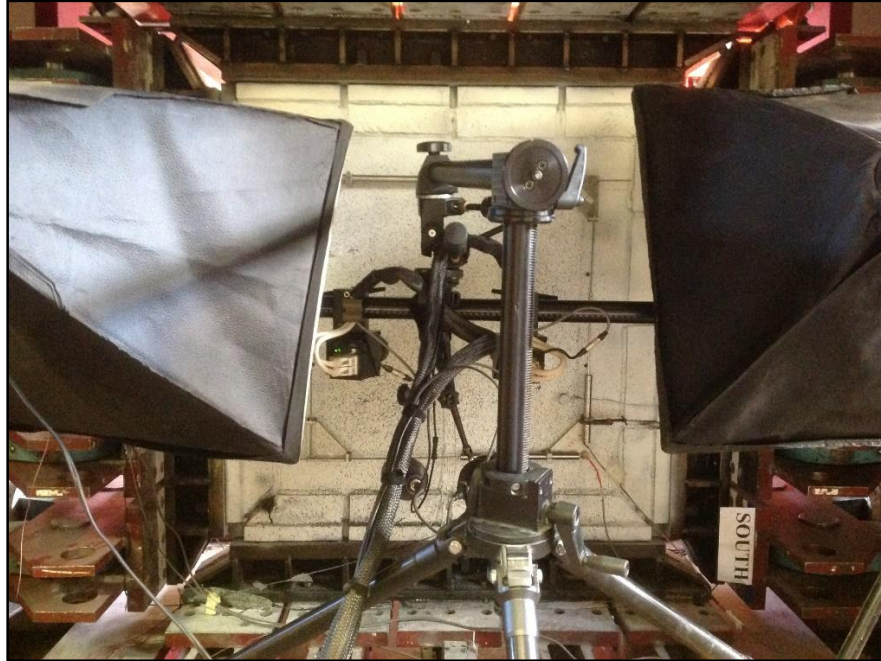
Figure 194. DIC setup on the south side
