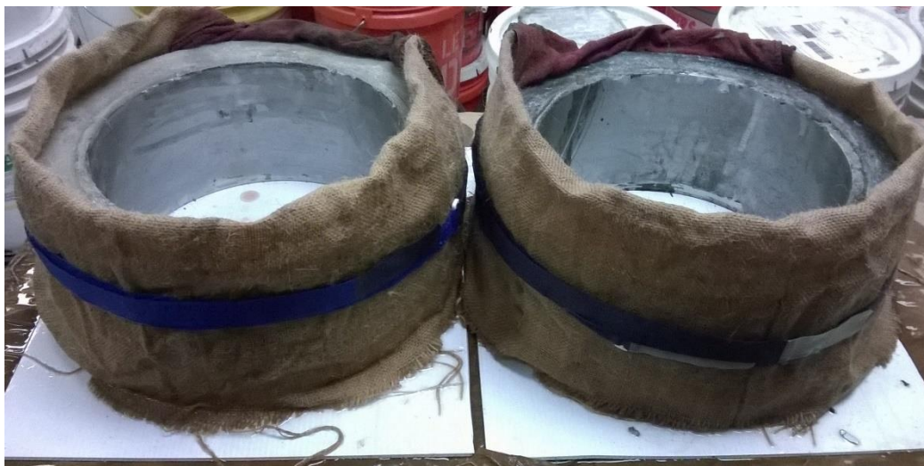
Figure 70. Three days wet curing to simulate field condition
