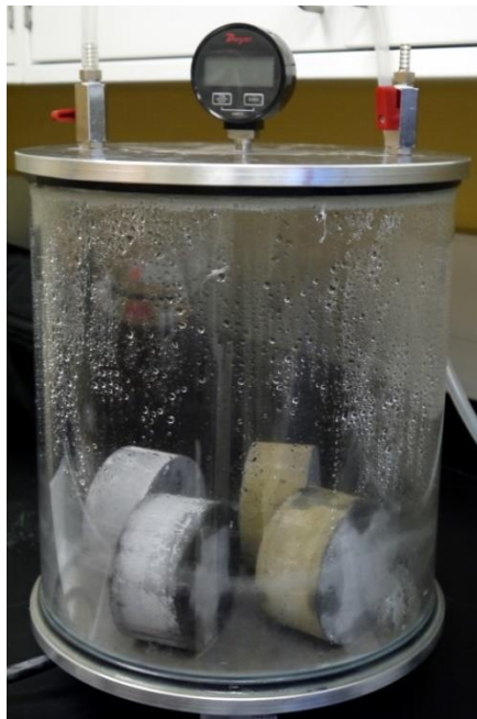
Figure 55. Conditioning of specimens with a vacuum desiccator
