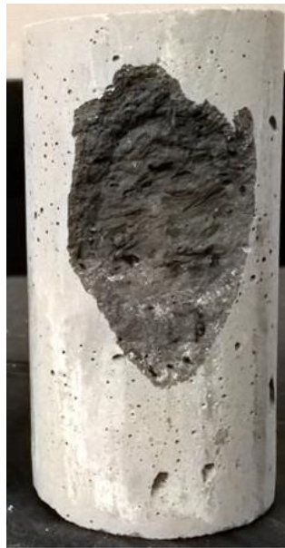
Figure 90. Locally spalled fiber-UHPC specimen at 350 °C
