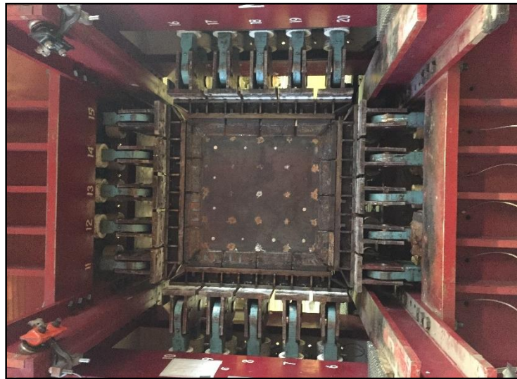
Figure 189. Fixing the wall panel inside the testing frame of UPT
