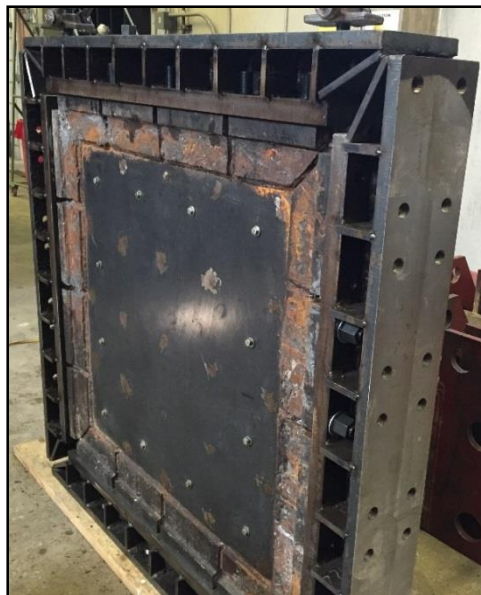
Figure 186. Setting up the steel beam frame onto the specimen
