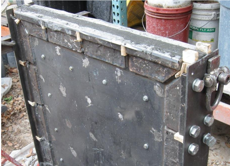
Figure 183. SC wall panel cast with UHPC
