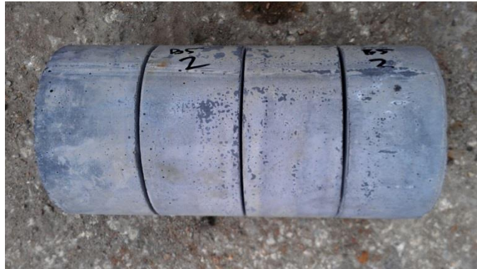
Figure 54. Cylinder specimens for rapid chloride penetration test
