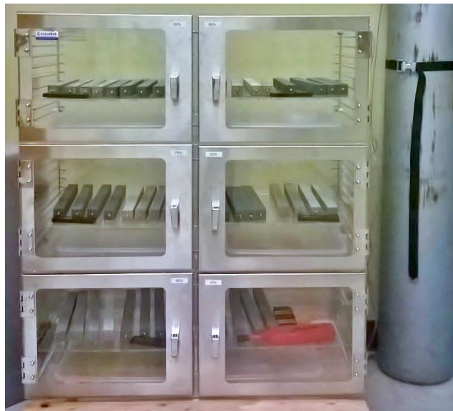
Figure 63. Controlled humidity desiccator for shrinkage at different RH
