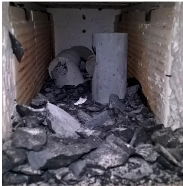
Figure 88. Furnace condition after heating at 400 °C
