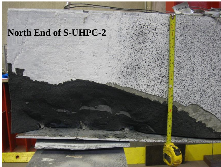
Figure 154. Spalling of concrete (S-UHPC-2 North)
