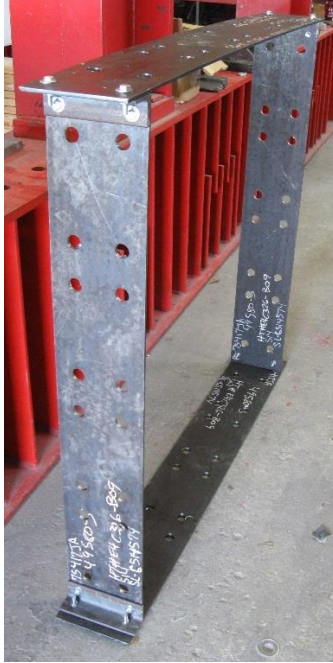
Figure 178. Steel formwork for test panel
