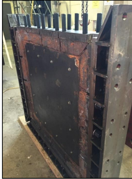
Figure 185. Inserting socket set screw bolts to the steel inserts
