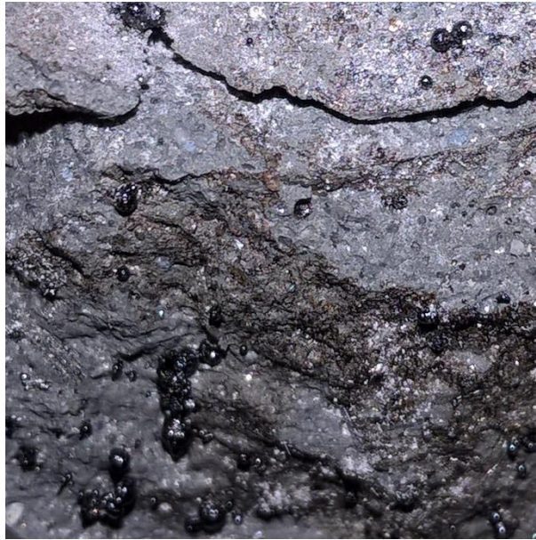
Figure 91. Appearance of decomposed fiber at 400 °C
