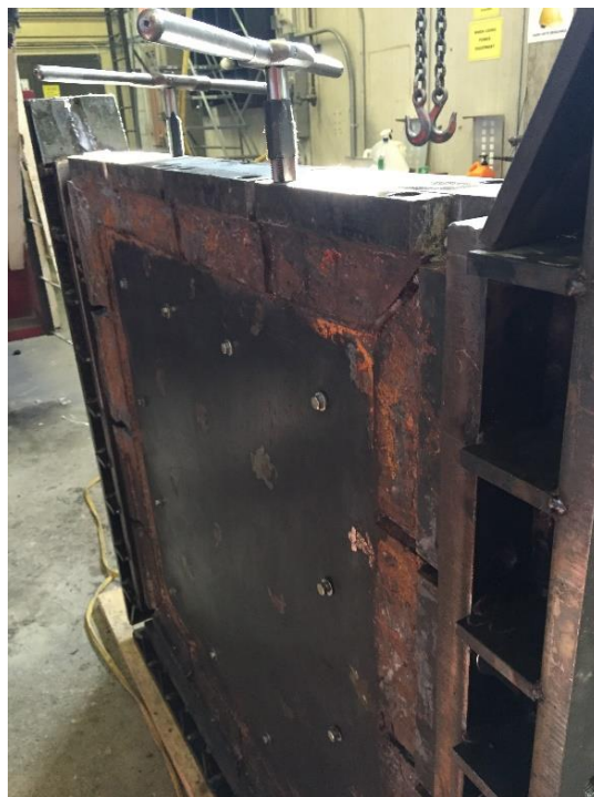
Figure 184. Tapping and cleaning the holes of the steel inserts
