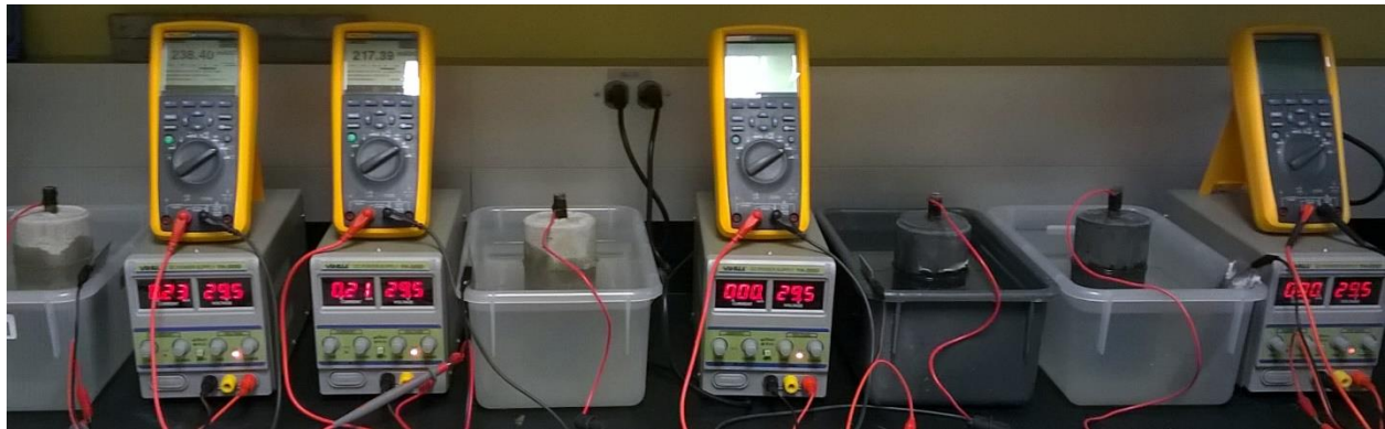
Figure 79. Corrosion test setup of UHPC and control concrete specimens
