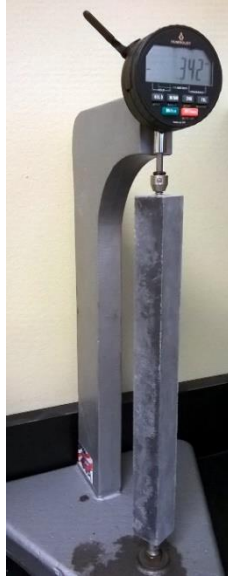
Figure 62. Test setup for free shrinkage measurement
