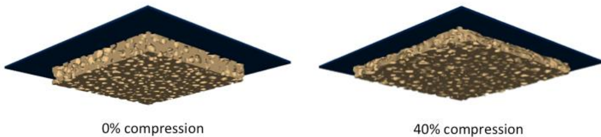
Fig. 20. Finite element modeling of a CT foam sample under uniaxial compression.
