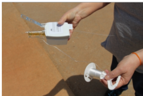
Radiosondes, like this one, are attached to weather balloons to collect vertical profiles (data sets) of both the thermodynamic state of the atmosphere and wind speed and direction.
