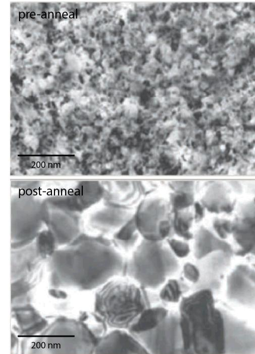
Ni that was initially nanocrystalline after exposure to 300°C for 30 minutes exhibits typical explosive grain growth
