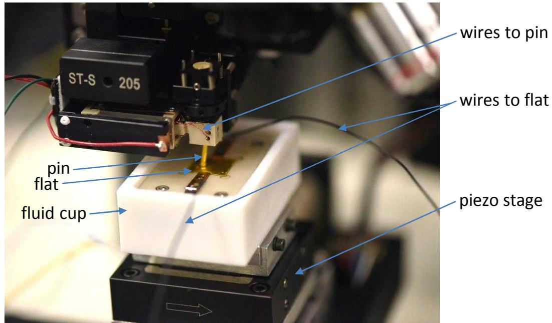
CSM nanotribometer modified for 4-wire ECR measurement
