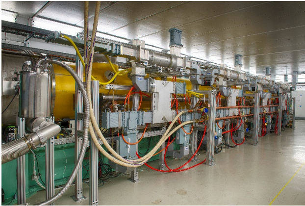
Figure 2: CM2 with waveguide distribution system.
