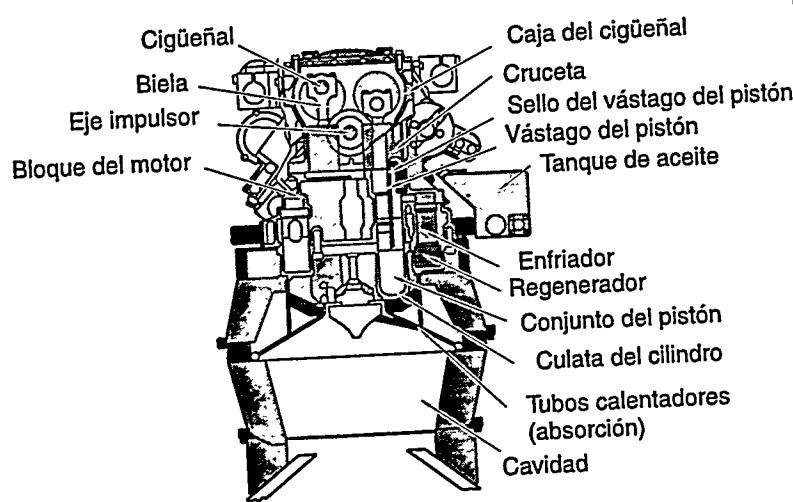
Fig. 4: Kinematic Stirling engine with a directly illuminated tube receiver
