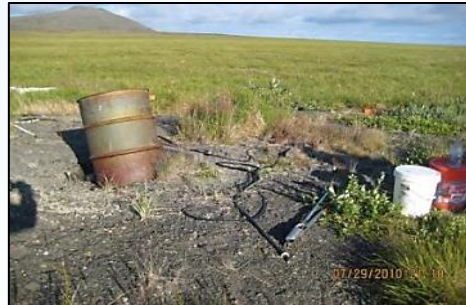
Test hole Baker with down-hole-temperature cable and sampling equipment
