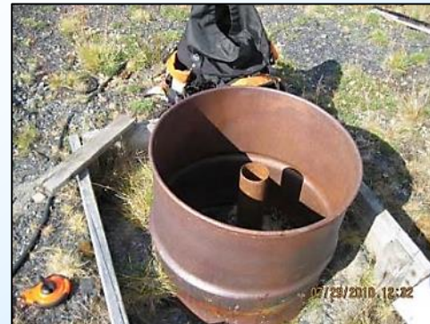
Test hole Baker with down-hole-temperature cable and sampling equipment
