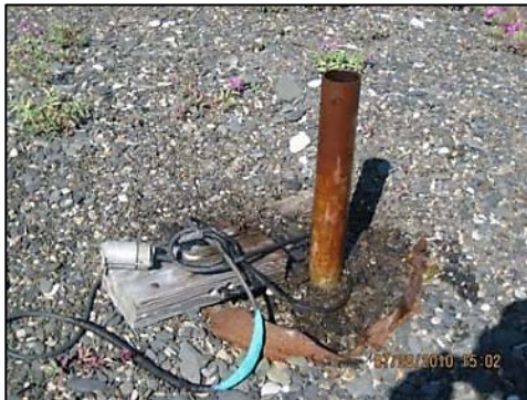
Test hole Baker with down-hole-temperature cable and sampling equipment
