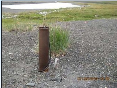
Test hole Able and down-hole-temperature cable
