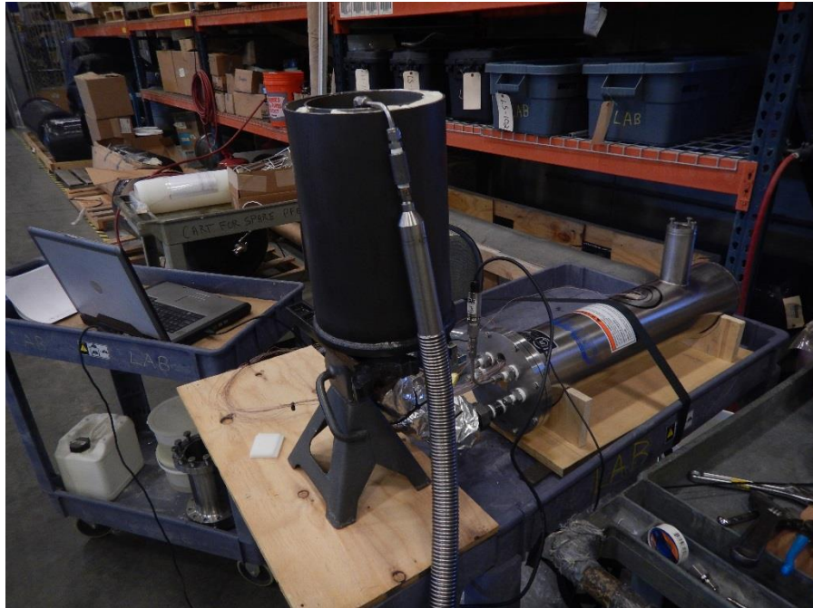
Figure 3.4.6: Front flood test setup
