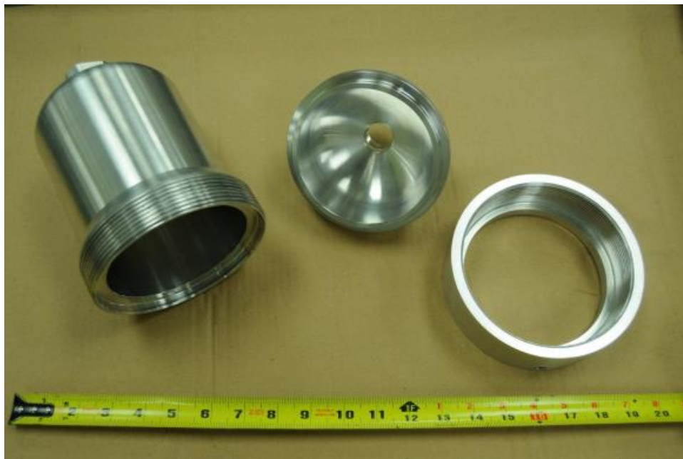
Figure 2.2.5: 3-piece Type 1 tank, disassembled
