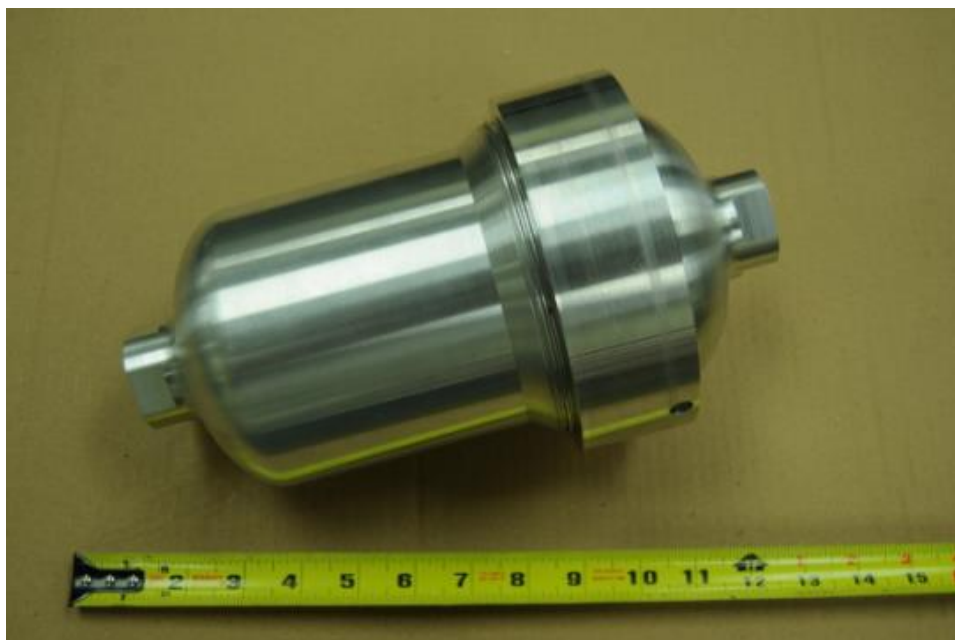
Figure 2.2.4: 3-piece Type 1 tank, assembled
