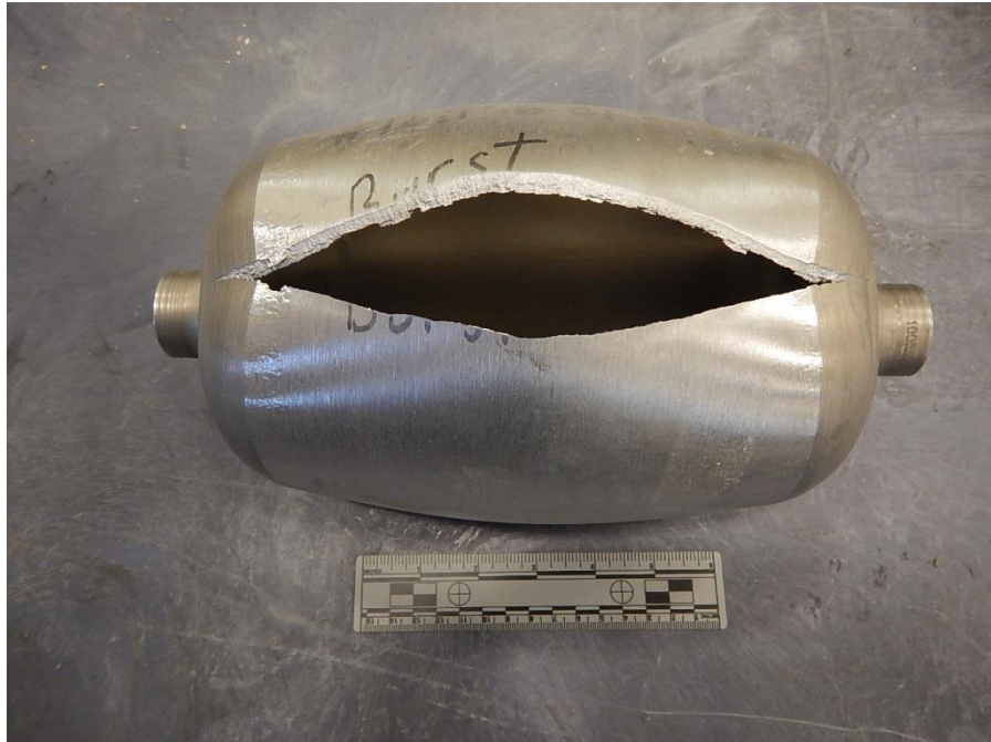
Figure 3.3.16: Type 1 tank after cryogenic burst test
