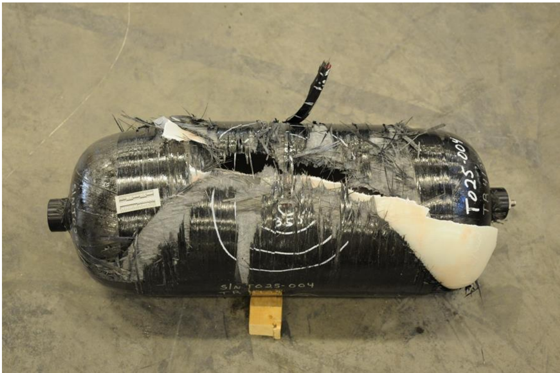
Figure 3.1.9: Tank burst after 350 J impact
