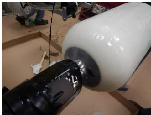
Figure 3.3.23: Braided cloth with liner resin on soluble mandrel
