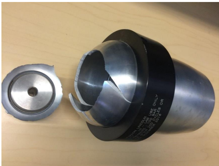
Figure 3.3.2: Test tank burst with LN2. Burst pressure was 380 bar
