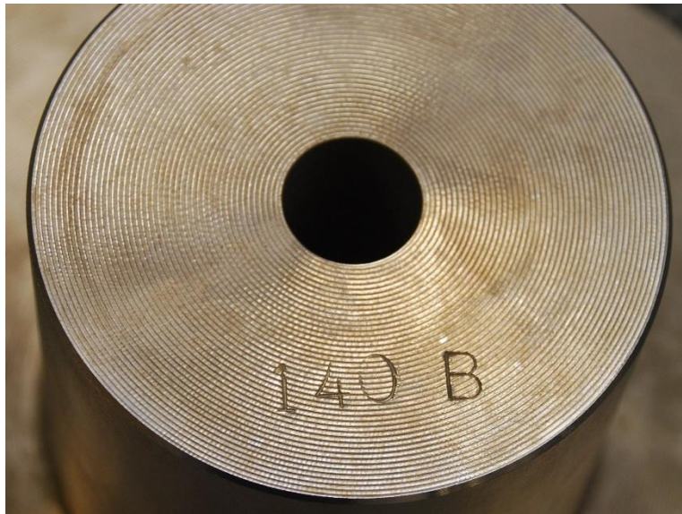
Figure 1.2.5: Near net shape 7075 aluminum boss with rough machined surface
