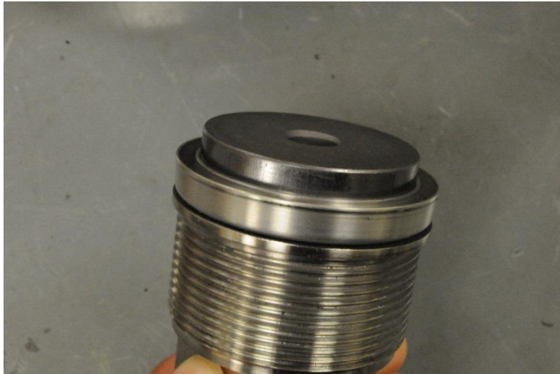
Figure 3.3.11: Aluminum cup seal installed on modified fitting
