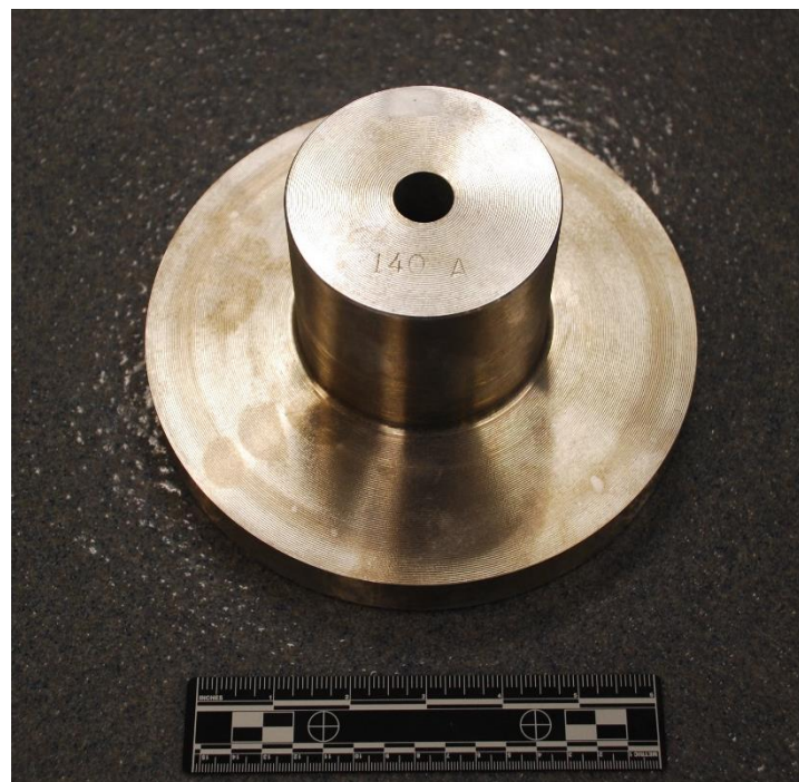
Figure 1.2.6: Example 7075-T73 near net shape boss
