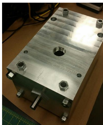
Figure 3.3.21: Assembled liner casting tooling
