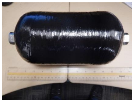
Figure 3.3.24: Completed tank with resin liner
