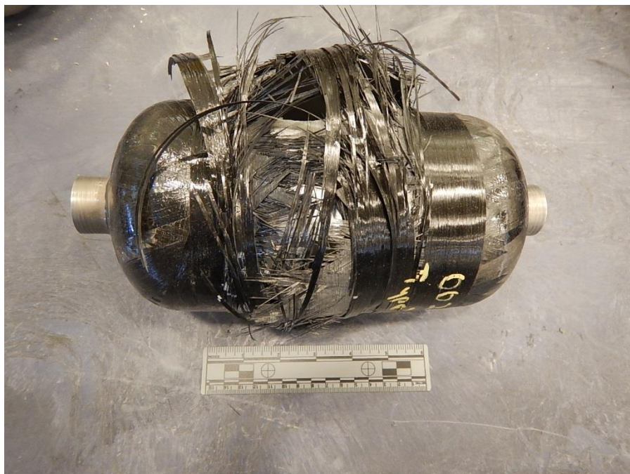
Figure 3.3.17: Type 3 tank after cryogenic burst test
