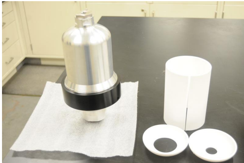
Figure 3.3.3: PTFE liner for the 3-piece aluminum tank next to it
