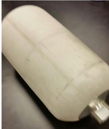
Figure 3.3.19: Cast mandrel from plaster
