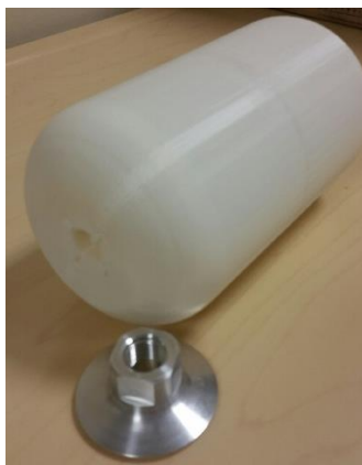
Figure 3.3.18: 3D printed mandrel
