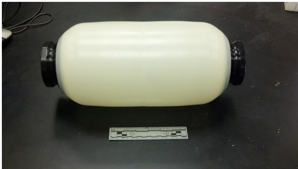
Figure 2.2.2: Liner used in the 6-liter Type 4 tank
