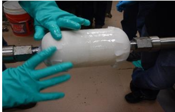
Figure 3.3.22: Polyester veil with liner resin on soluble mandrel
