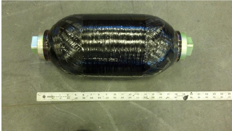
Figure 2.2.1: 6-liter Type 4 pressure vessel
