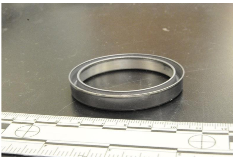
Figure 3.3.10: Aluminum cup seal for the large port
