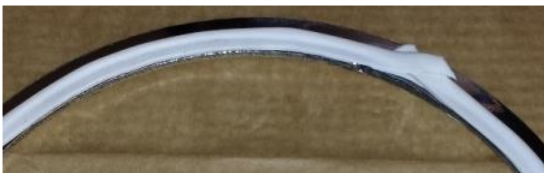
Figure 3.3.7: Teflon sealant on large aluminum seal before compression
