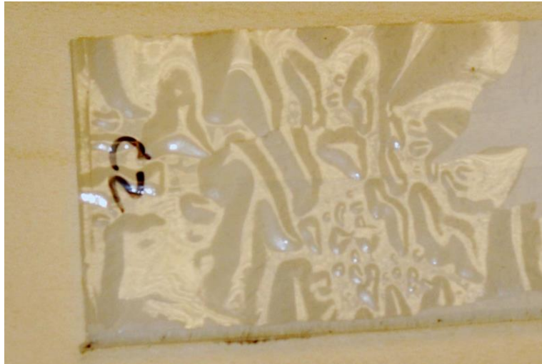
Figure 1.2.2: Example of PVDC coating peeling away from an HDPE substrate after hydrogen saturation
