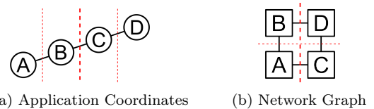
Figure 10: Example for mismatching coordinates and allocation. The dashed lines represent the bisection cuts.
