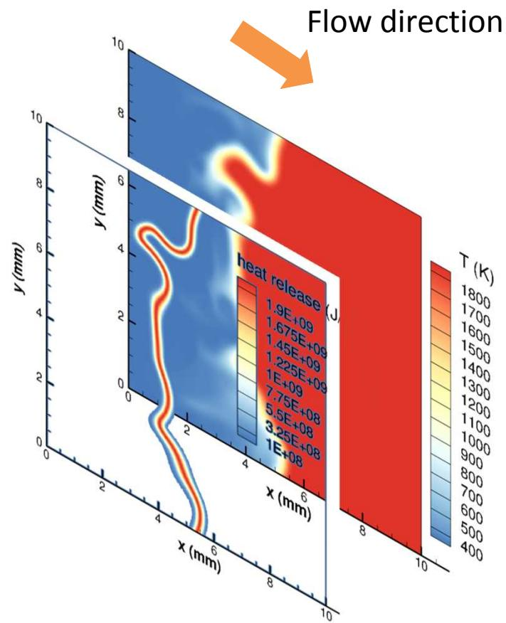
A lean ( $\Phi=0.7$ ) premixed methane flame is simulated using DNS (s3d).
