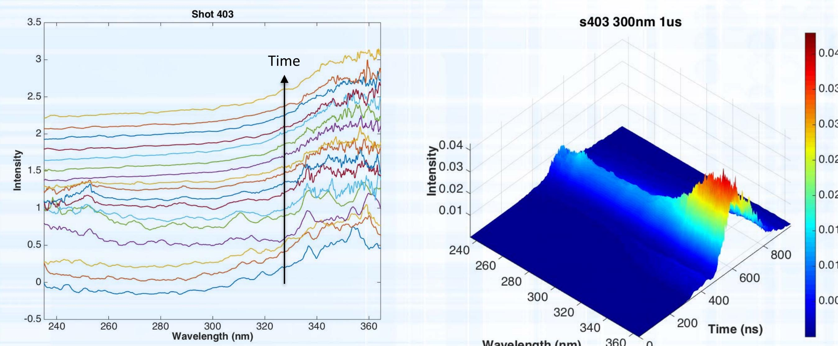
UV emission from detonating PETN, 300 nm center: (left) time resolved spectra, 25 ns increments. (right) spectral surface-map.
