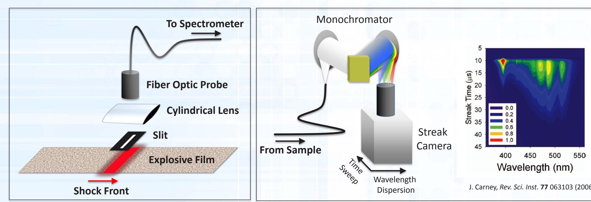
Diagram of the spectroscopy experiment. A detonation proceeds laterally through a vapor deposited film of explosive (PETN, HNS, HNAB). Light emission is captured, spectrally separated, and recorded by a streak-camera.
