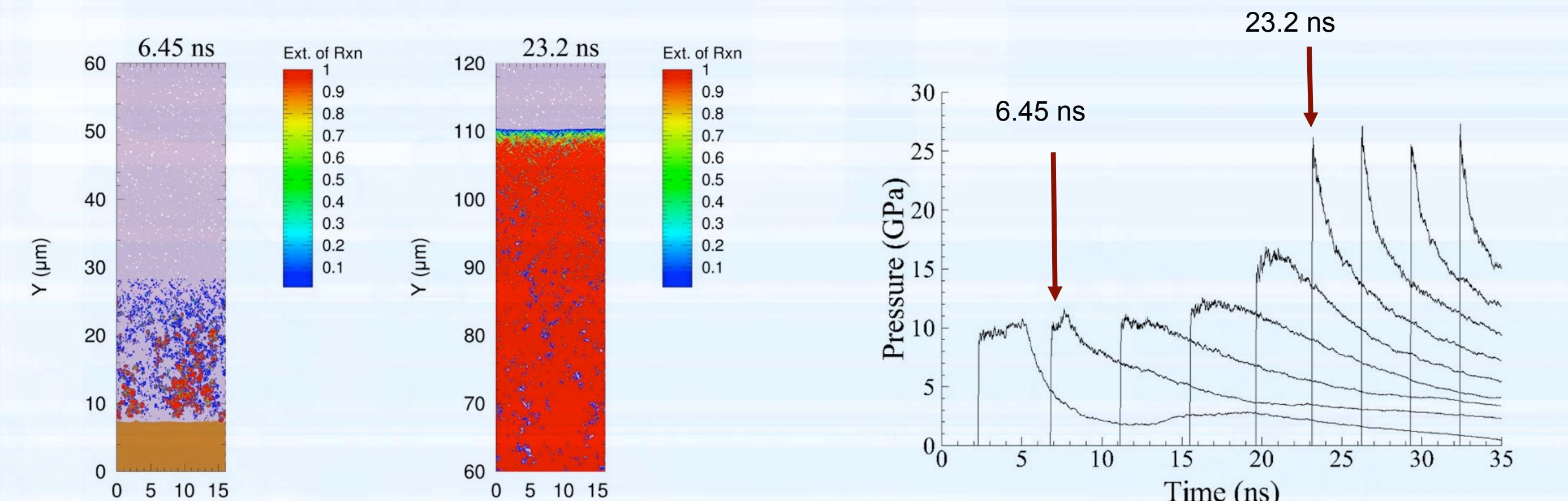
Grain-scale simulation of HNS initiation. (left) extent of reaction at 6 and 23 ns after flyer impact. (right) pressure histories showing build-up to detonation
