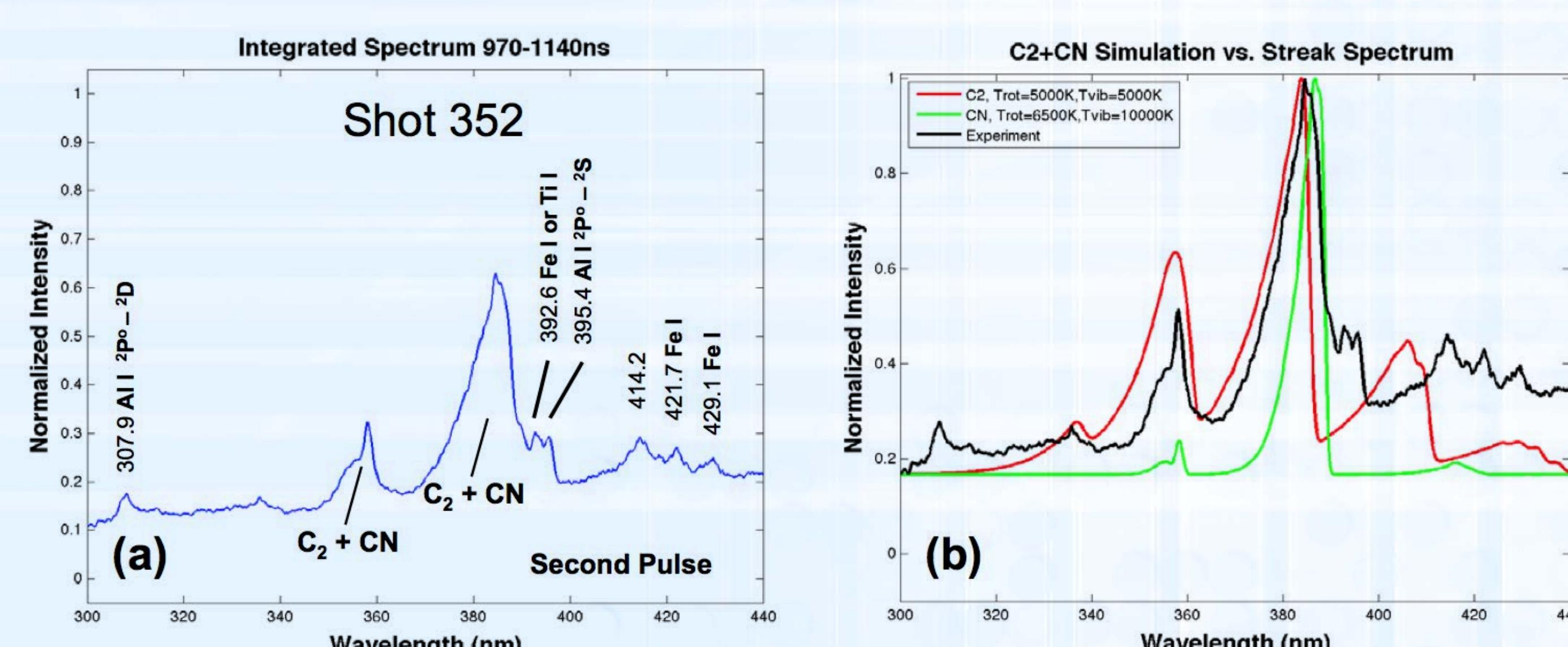
UV emission from detonating HNS, 380 nm center: (a) integrated spectrum and (b) comparison with simulated emission spectra from C2 and CN.
