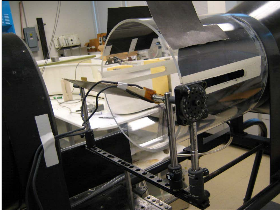
Figure 3.5-10 Airfoil model in the wind tunnel
