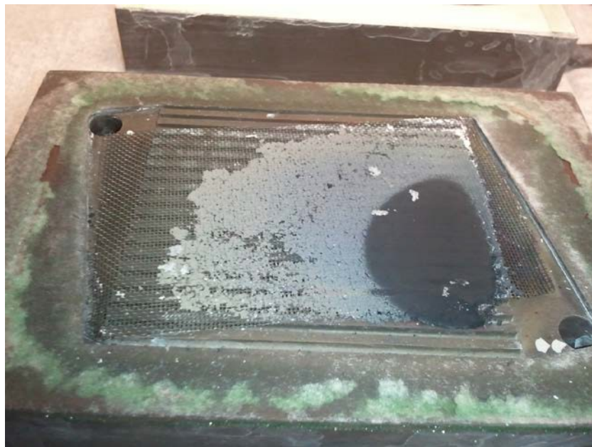
Figure 2.3-1. Soot formation under \text{CH}_4 in a NextCell due to insufficient water vapor.
