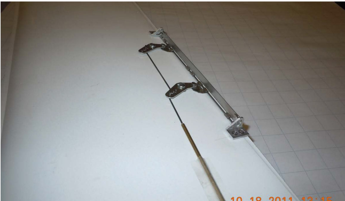
Figure 3.5-18: Lab prototype of the Gurney flap mechanism
