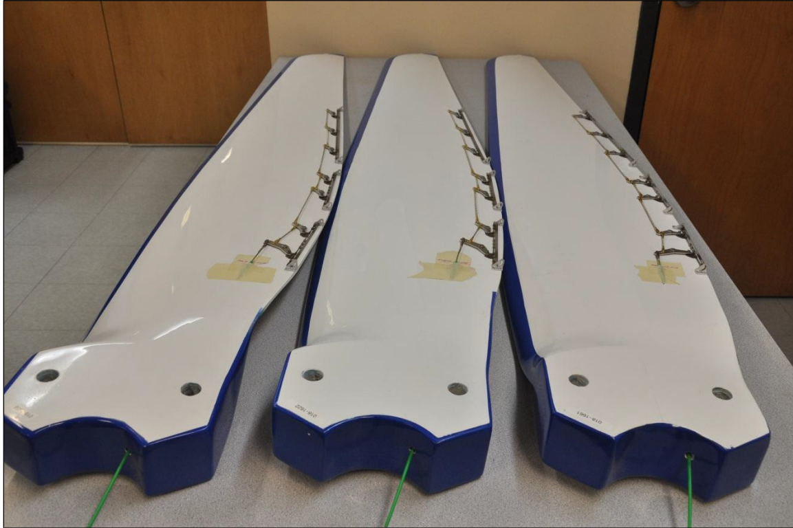
Figure 3.5-21 – ARE 110 Wind turbine blades with Gurney flap mechanisms installed on their trailing edge.
