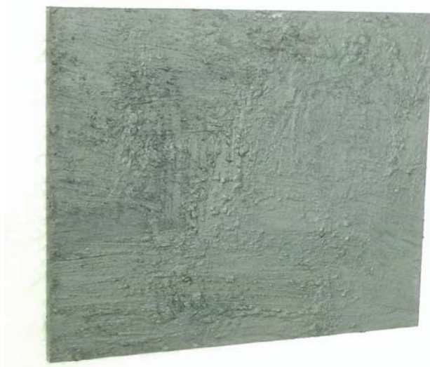
Figure 2.4-13. Acrylic flat painted with a mixture of platinized \text{MoS}_2 and Teflon.
