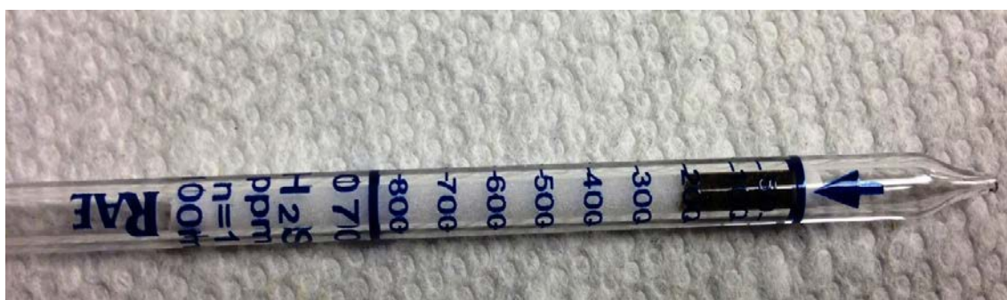
Figure 2.4-12. H 2 S concentration in landfill gas detected by RAE tubes
