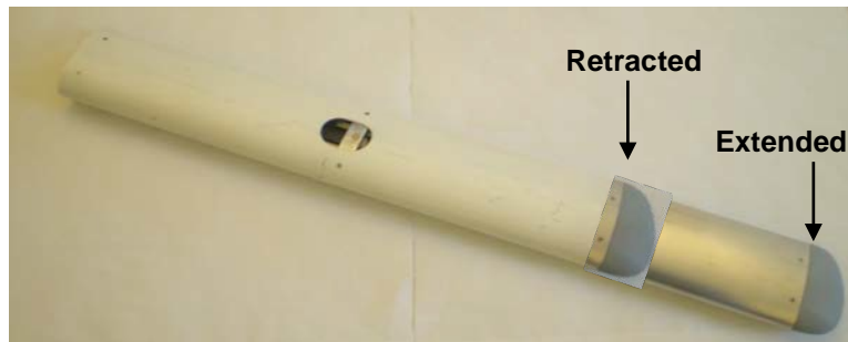
Figure 3.5-14b: Photo of Variable Radius Blade mockup – Retracted & Extended
