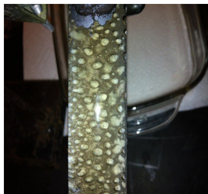
Figure 2.4-5. Bubbles of hydrogen gas on Teflon strip.
