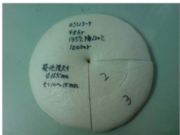
Figure 4. ISTN3-9. Foamed at 121°C, 110 bar. Foam diameter 165mm.
