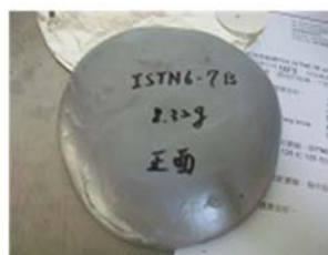
Figure 8. ISTN6-7B: Foaming T 123°C, Slower (3 sec) gas discharge, Density 33kg/m 3
