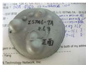
Figure 7. ISTN6-7A: Foaming T 123°C, Density 258 kg/m 3
