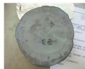
Figure 8. ISTN6-7B: Foaming T 123°C, Slower (3 sec) gas discharge, Density 33kg/m 3
