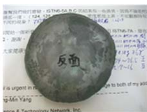
Figure 7. ISTN6-7A: Foaming T 123°C, Density 258 kg/m 3
