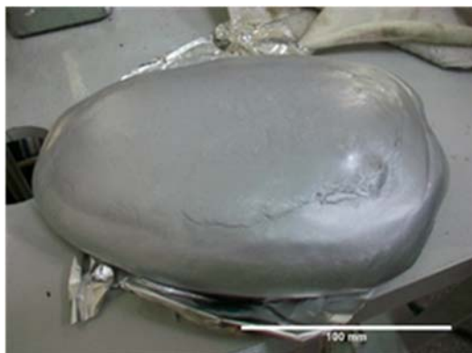
Figure 9. ISTN3-8 with 1.9% Al additive. Foam density = 33 kg/m 3 Aged R value/in = 4.55.
