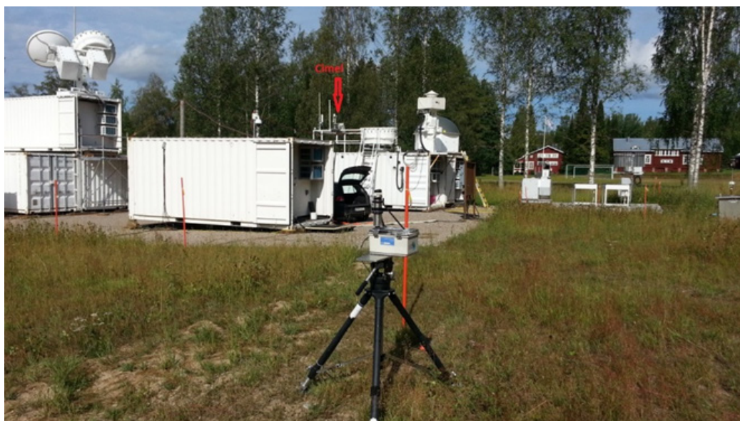
Figure 2. TWST sensor location, shown here on the tripod in the foreground, in relation to other cloud and aerosol sensors during BAECC campaign. The Cimel sun photometer used for the AERONET sensor is indicated in the figure by a red arrow. The TWST computer is located in the white seatainer behind and to the left of the TWST optical head.
