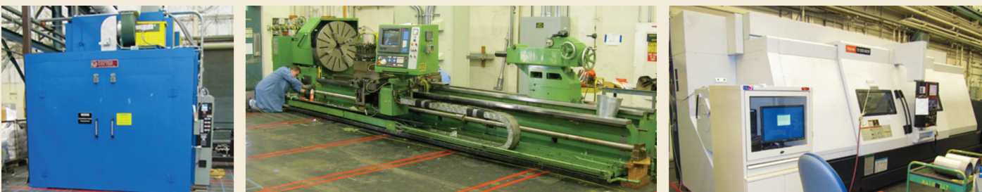
Figure 2. The curing oven (left), large turning lathe (center), and five-axis machining center (right) were acquired to support the BLU-129/B project.
