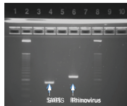
Figure 3. Agarose gel image showing bands for SARS and Rhinovirus amplicons proving that the recovered DNA was undamaged and could be analyzed.
