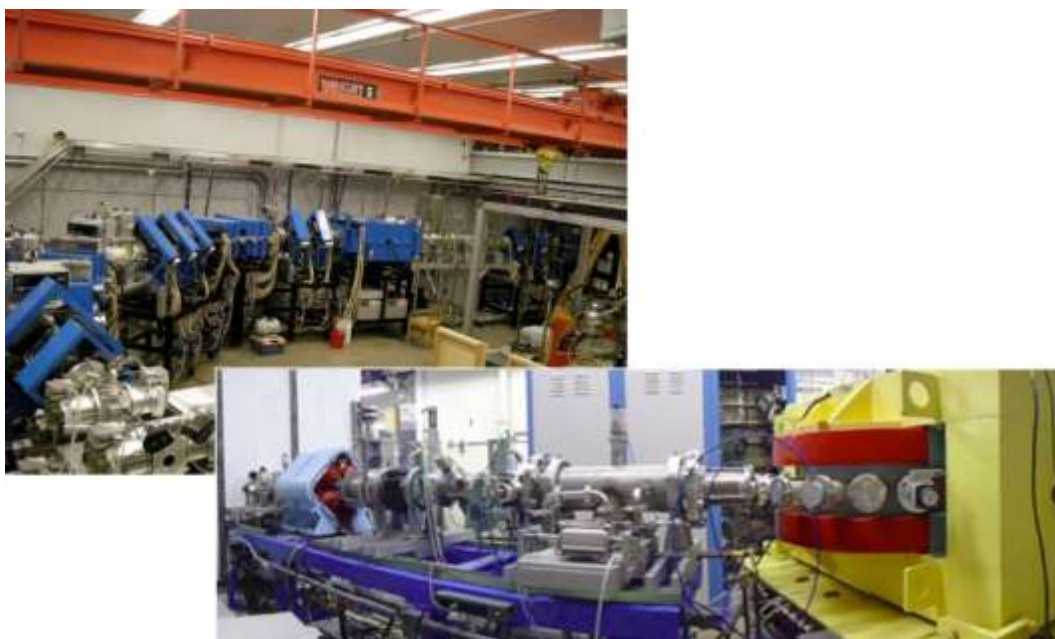
Figure 19: University accelerator facilities, organized in the ARUNA network, provide stable, neutron, and gamma beams that are critical for measurements of astrophysical reactions that involve stable nuclei and govern the evolution of stars. (Upper left: University of Notre Dame Nuclear Science Laboratory, Lower right: LENA accelerator at TUNL, Credit: Christian Iliadis)
