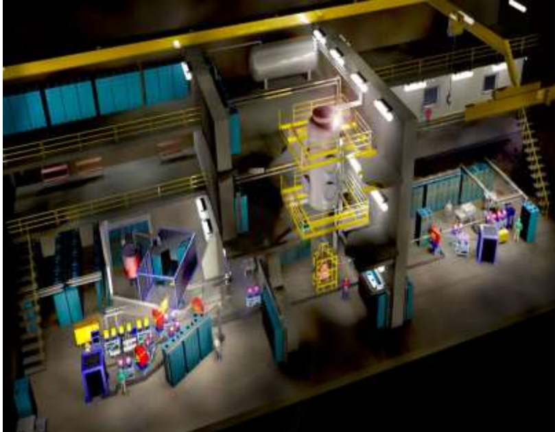
Figure 20: A low energy underground accelerator for intense stable beams is a high priority for nuclear astrophysics. The cosmic ray background shielding provided at an underground location enables measurements of very slow astrophysical reaction rates at, or very close to astrophysical energies. (DIANA concept study).
