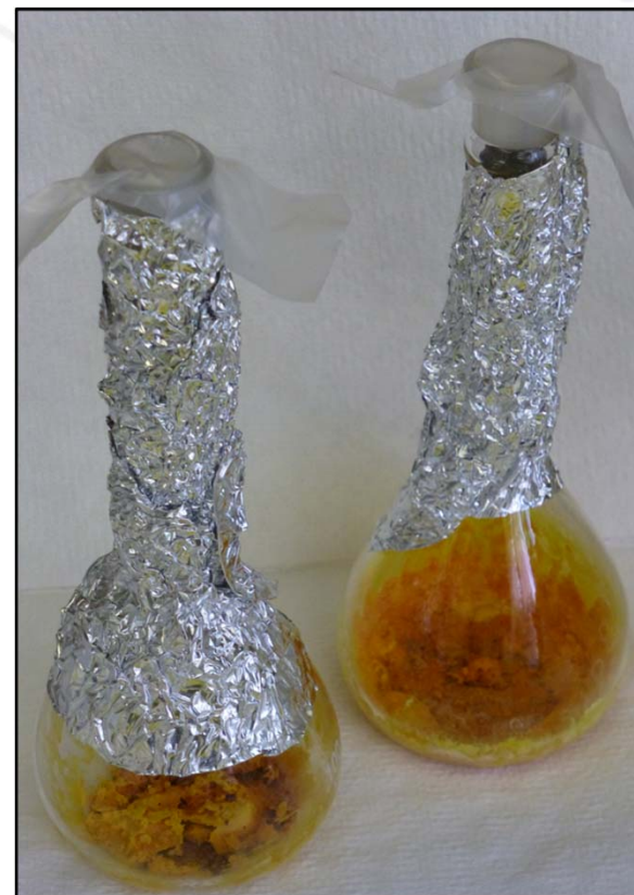
Picture shows \text{UO}_3 \cdot x\text{H}_2\text{O} formed during preparation of solns. 11 & 12
