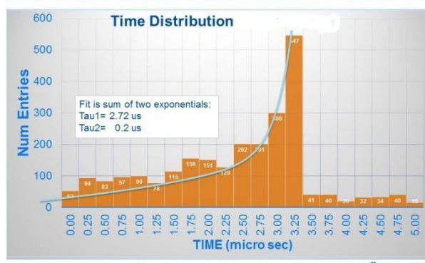
Figure 7. Time distribution of the scintillation counter signal. Notice the presence of a fast and a slow component.
