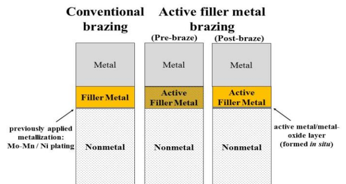
Figure 1. Schematic showing conventionally brazed and active filler metal brazed metal/nonmetal sample.
