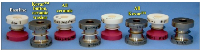
Figure 19 Photograph shows the variants of the tensile button samples.
