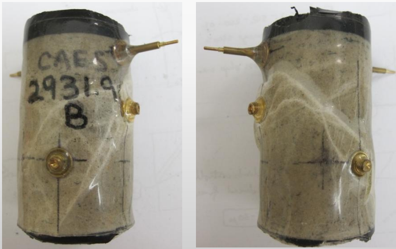
Laboratory shear bands in weak Mt Simon Facies
