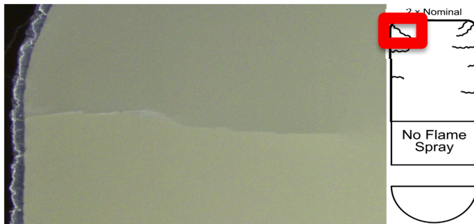
Figure 9: Optical microscope image of a cohesive crack near the top right fillet of the twice nominal cylinder taken to 155° C.
