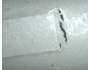
Figure 2: (a) A photo of cracks in front of the copper strip that penetrate into the epoxy substrate, and (b) a photo of the cracks in the flame spray of the epoxy cylinder that was taken to -55^{\circ}\text{C} 60 times.
