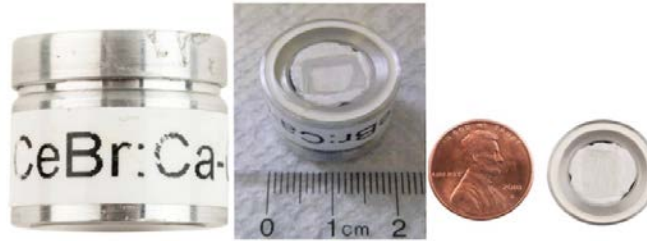
Fig. 1. Packaged scintillator of 0.2 atomic% \text{Ca}^{2+} -doped \text{CeBr}_3 .
