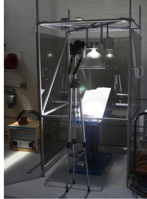
Figure 12. Flux mapping with a camera and a white board at 30^\circ tilt angle
