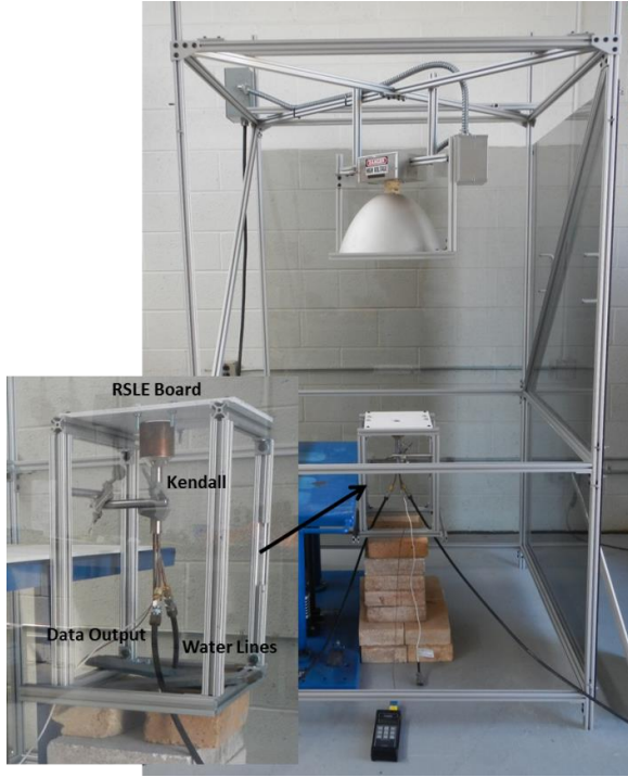
Figure 11. Kendall radiometer mounted on a holding system for irradiance calibration measurement
