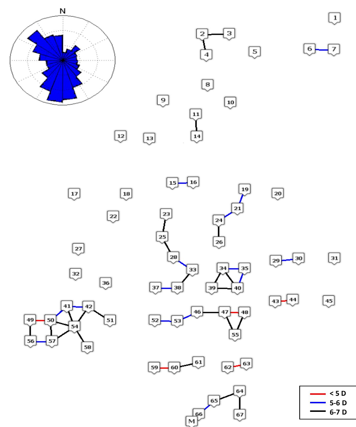
**Visualizing Wake Effects.** After data correction (including met tower wind direction, nacelle wind direction, and power curve based on pitch schedule), a method for visualizing wake effects was developed called *normalized instant power*. For turbine  $i$ , the *normalized instant power* is defined to be
