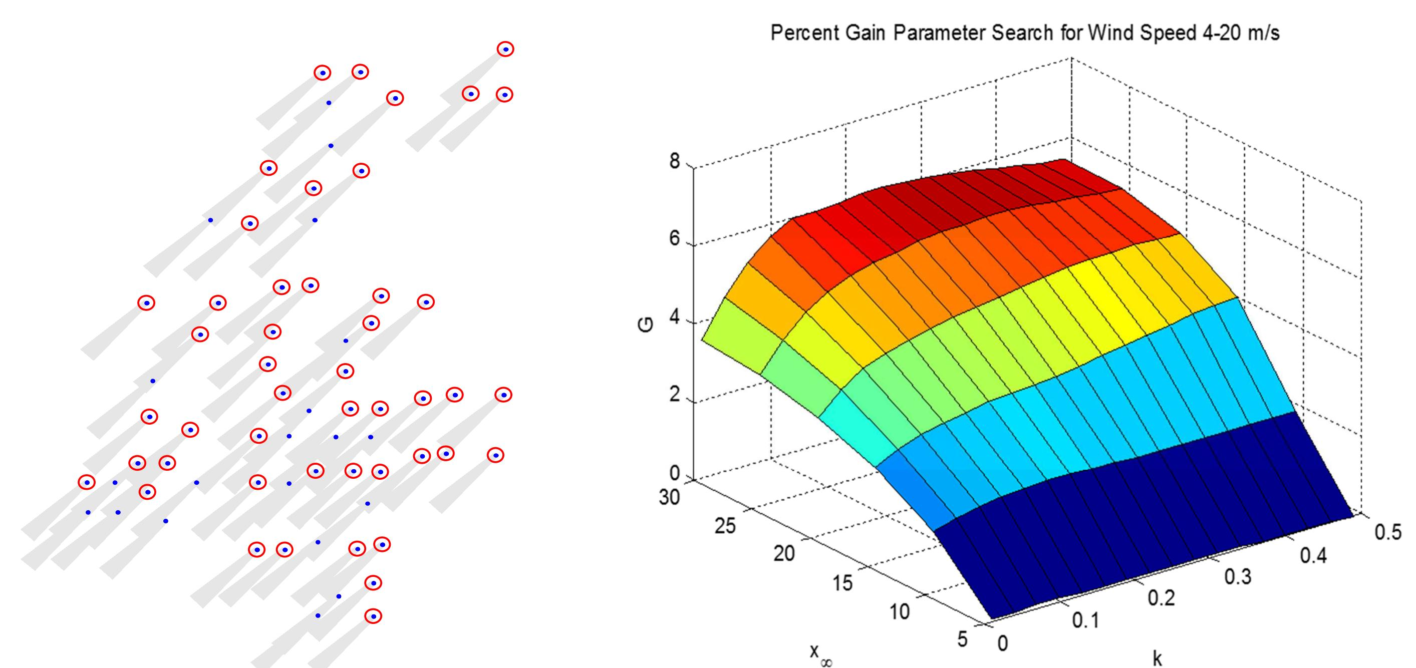
**Conclusions.** Using visualizations, three wake effects were observed: deficits, speed up channels, and shear point speed ups. In some cases, the speed ups serve to mitigate the wake deficits.
