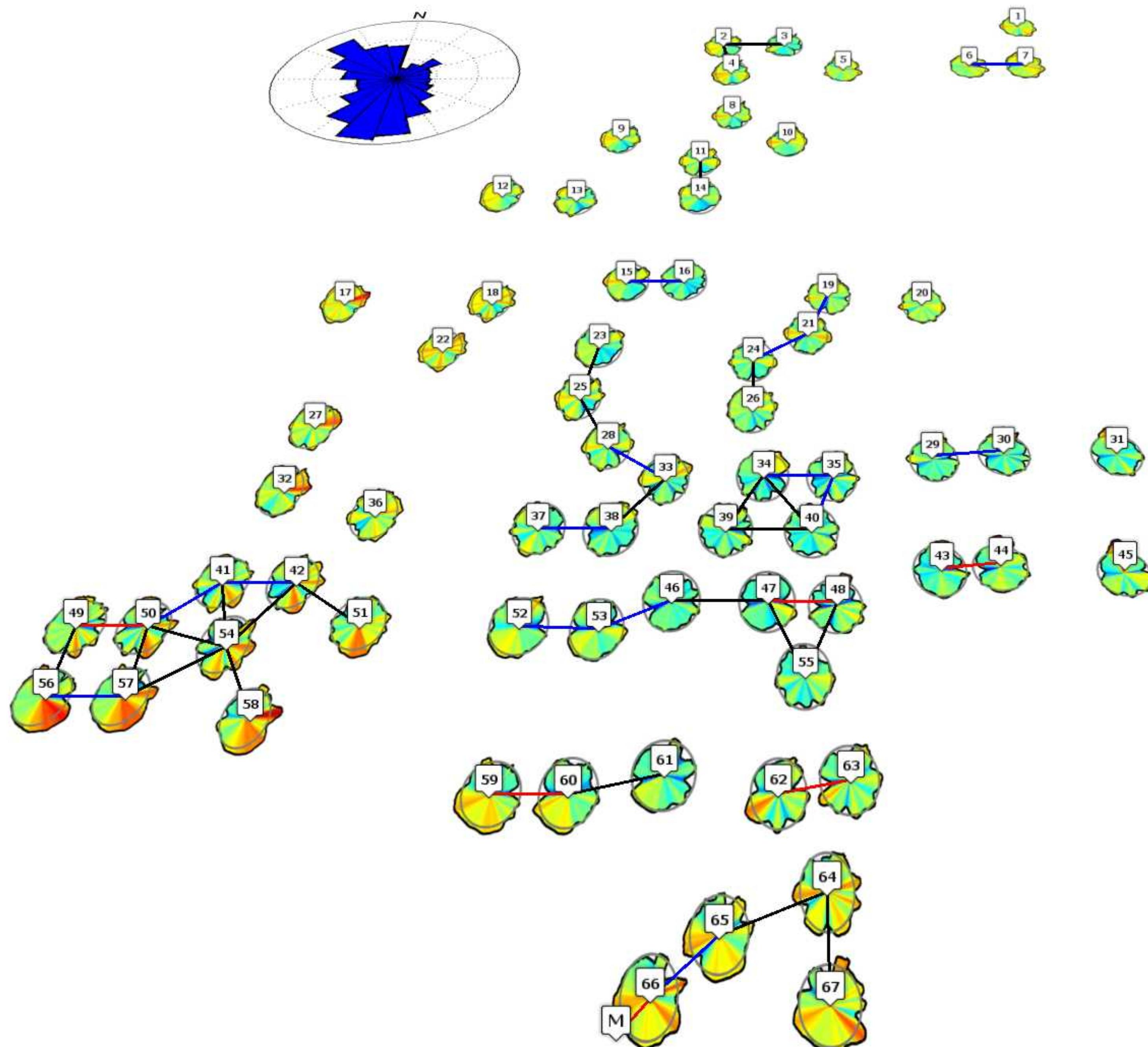
**New Wake Effects.** In addition to providing an overview of the wind farm, the normalized power and power variability plots can be used to understand wake effects on a more detailed scale. Four distinct features have been observed in the data:
