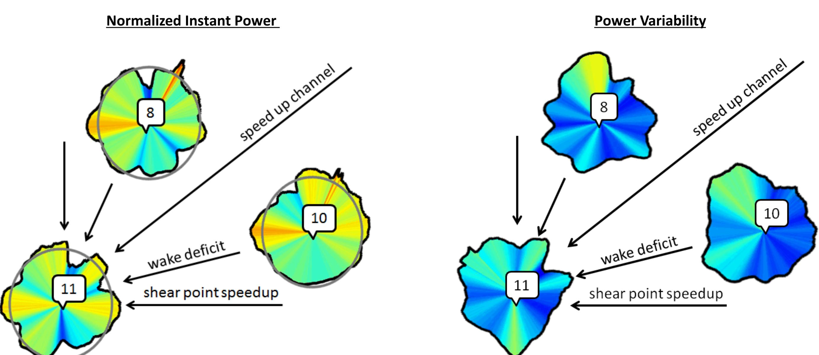
**Quantifying Wake Losses.** To estimate power lost due to wake effects, an approximation of the wind speed in the absence of upwind turbines needs to be computed. This can be done if the upwind turbines throughout the farm are identified and used to extrapolate the true wind speed for the shadowed turbines. Shadows were computed using the Park model [1]
