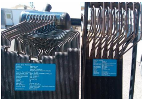
Figure 1: a) Solar One Receiver (1981-1987) was a Water/Steam Receiver with thermal rating of 41 MW (175-516°C at 10 MPa) and b) Solar Two Receiver (1996-1999) was a Nitrate Molten Salt Receiver with thermal rating of 42.2 MW (288-566°C at ~2 MPa).
