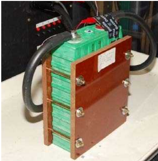
International battery Li-ion \text{FePO}_4 large format prismatic 160 Ah cells
